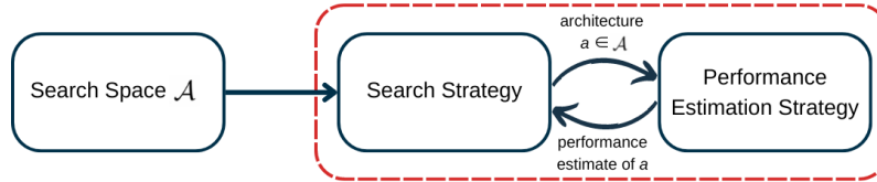
Figure 2.3: NAS dimensions [EMH19]: A search strategy iteratively picks architectures from a predefined search space \mathcal{A} . The chosen architectures are assessed by a performance estimation strategy, providing performance estimates back to the search strategy.
