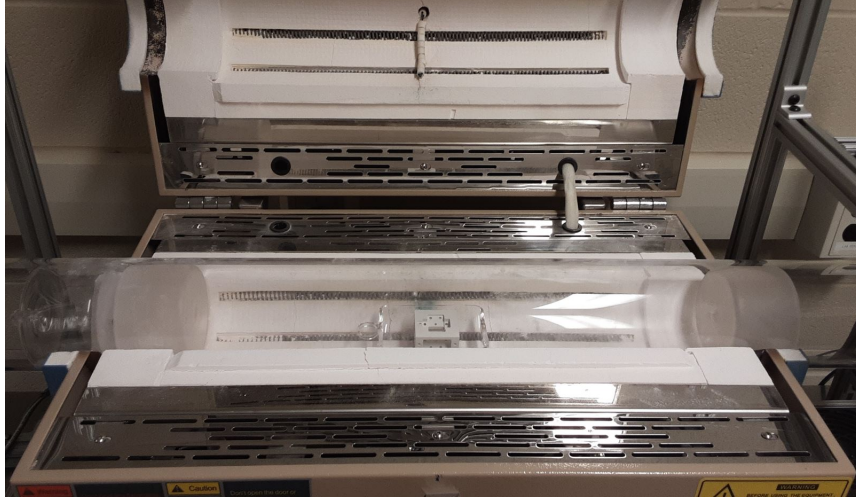
Figure 5.31: High-Temperature Prebake of Shapal Ion Trap Mount
