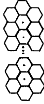
Fig. 6.4. Configuration for hexagonal cells in a VCT with the maximum value of p
