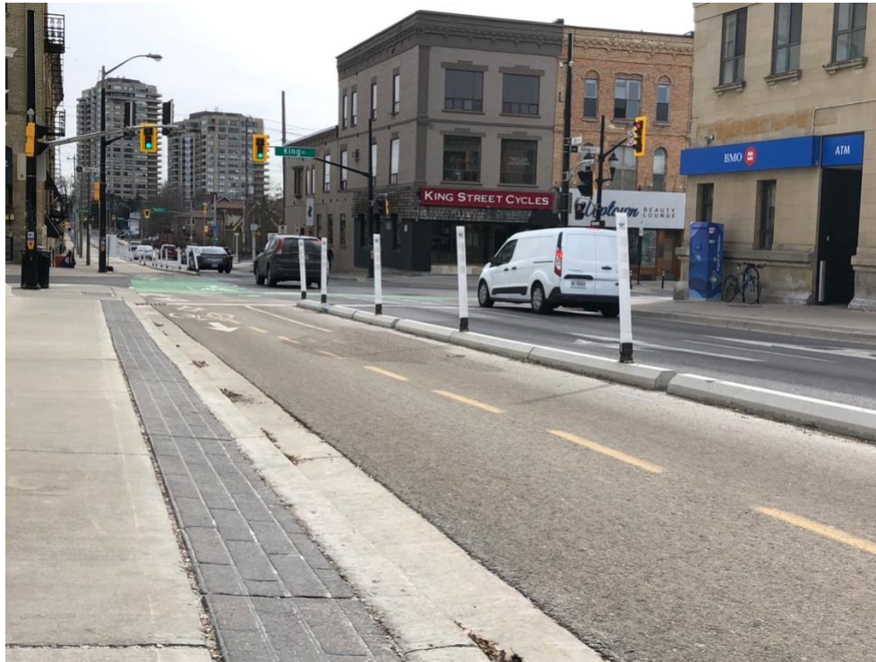
Figure 1.6: A Stretch of New Cycling Lanes that Were Implemented by Removing a Lane of Traffic
