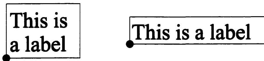
Figure 2.3: Using an elastic label to set a text label.
