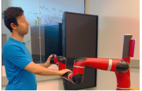
Figure 1.2: Example of a direct pHRI application: a user exercises with a collaborative robotic arm by pushing against its stiff joints.
