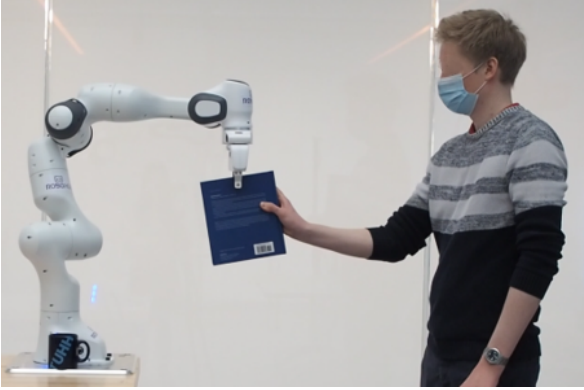
Figure 1.1: Example of an indirect pHRI application: a collaborative robotic arm mediates the interaction between the user and an object, such as handing over a book.
