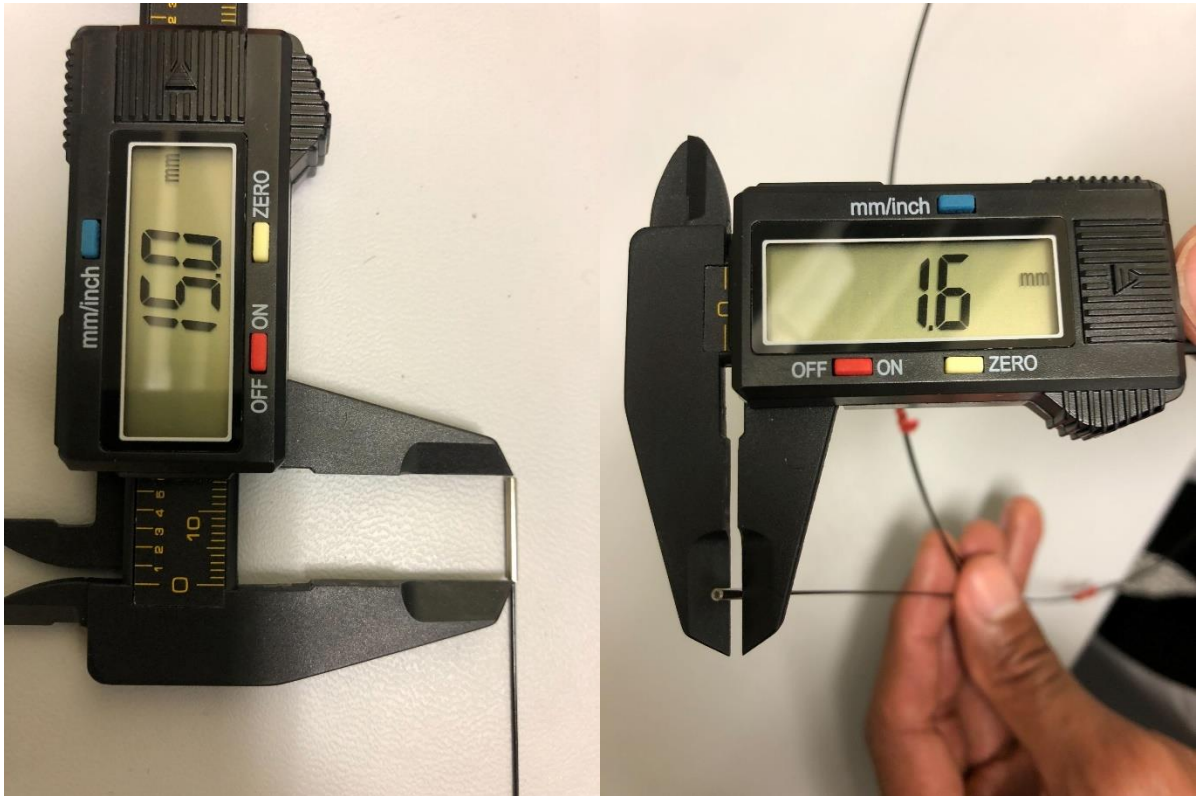
Figure 18: PARS P1 EM distal end showing critical dimensions of GRIN lens assembly
