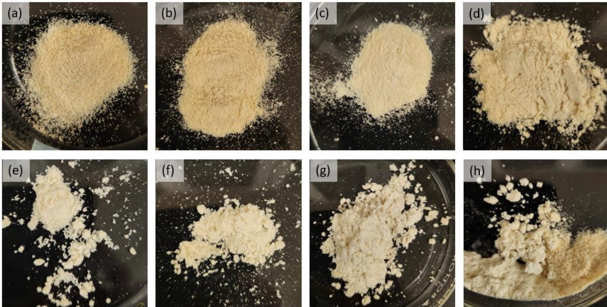
Figure S. 2: Visual observation of the color difference between the various size fractions of dried okara obtained through filtration (a) > 212 μm (b) 212 - 106 μm (c) 106 - 75 μm (d) 75 - 63 μm (e) 63 - 45 μm and (f) < 45 μm; (g) Color difference between okara particles of size >212μm and <45μm.
