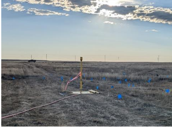
Figure 2-3: Modular stack configured for releases from 1.7m above the ground
