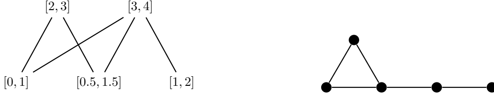
Figure 1.4: The Hasse diagram of the unit-interval order on intervals \mathcal{I} = \{[0, 1], [0.5, 1.5], [1, 2], [2, 3], [3, 4]\} (left) and the incomparability graph of this poset (right). This corresponds to the natural unit-interval order P(3, 3, 4, 5) .
