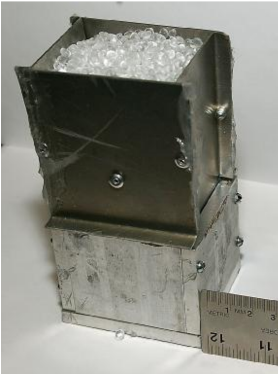
Figure 4.5: Hopper filled with Elvax® pellets placed on top of the mold (i.e. step 3).
