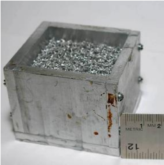
Figure 4.4: Assembled and lubricated mold with an aluminum foam specimen placed inside (i.e. step 2).
