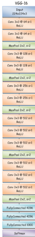
Figure 4.3: VGG16 architecture from Simonyan and Zisserman (2014) , characterized by uniform 3 \times 3 convolutional kernels and deep sequential blocks. Block diagram modified from Mora et al 2020 [28]
