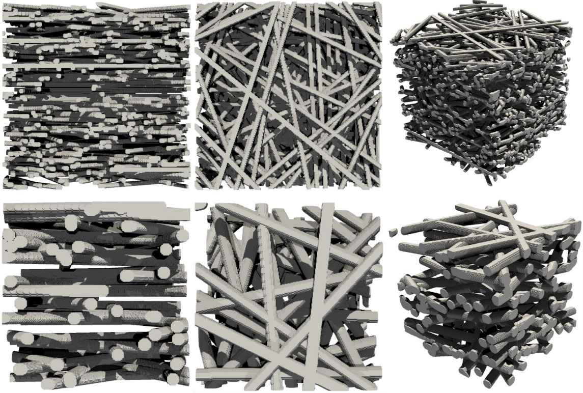
Figure 9 – Sample images of fibers randomly oriented in the x-y plane but aligned along the z axis. Top row shows structure containing more fibers with small diameter, while bottom row shows structure containing fewer fibers with larger diameter. Images with n = 100 \rightarrow 600 and r_f = 3 \rightarrow 20 were evaluated.
