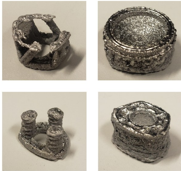
Figure 3-16 Melting of Ti64 devices during the EBM process with experimental melt theme.
