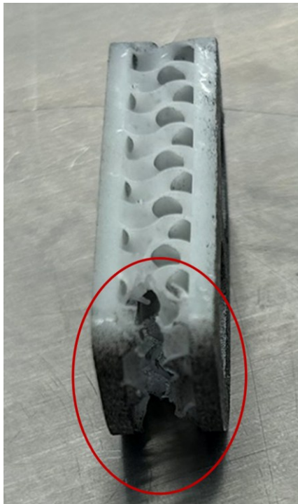
Figure 4-19 Flat latticed implant failure of the lattice under compression at around 450N. The edge, circled red in the figure, where the implant contacted the Sawbones, experienced brittle failure. The test was stopped after failure.
