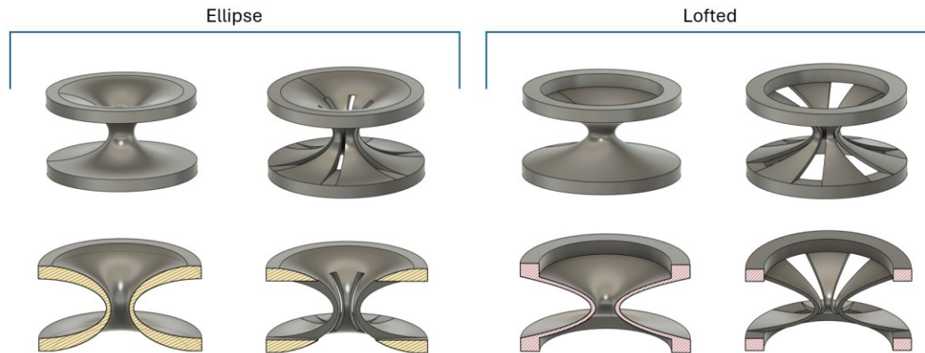
Figure 3-3 CAD of the device geometries for the spindle like design with a section cut view on the bottom. Left to right: ellipse, ellipse with 1 mm slits, lofted, lofted with 2 mm slits.
