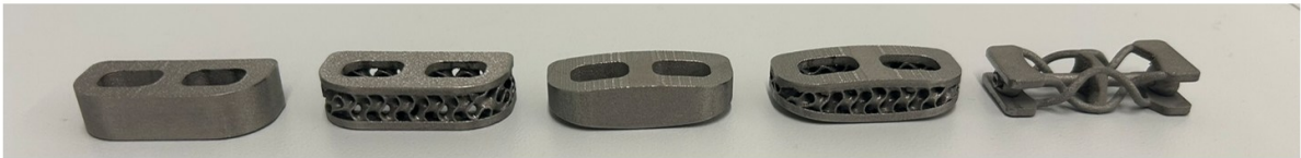
Figure 4-18 The five implant specimens. The implants printed in Rigid 4000 are shown on top and are speckled. The bottom implants are the metal AM printed Ti64 implants. The implant types from left to right: flat, flat latticed, anatomic, anatomic latticed, and DSCI. In the resin set the additional DSCI (rightmost) is made from tough resin.
