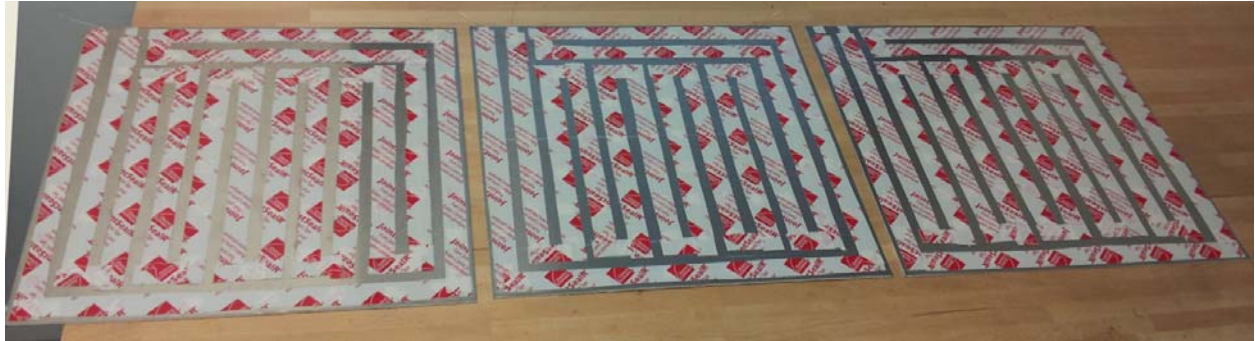
Figure 11 – Taped heater wire on the back of the meter plate and side guards.
