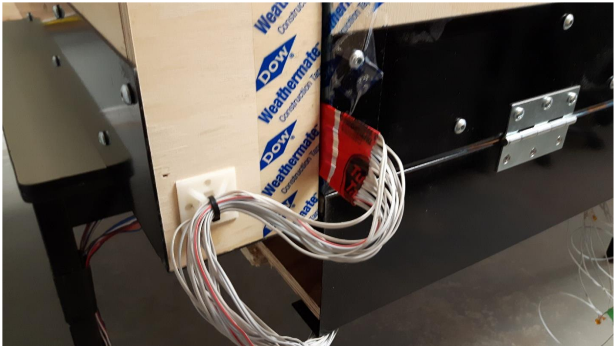
Thermistors from the hot plate assembly coming out of the apparatus in-between the edge insulation.
