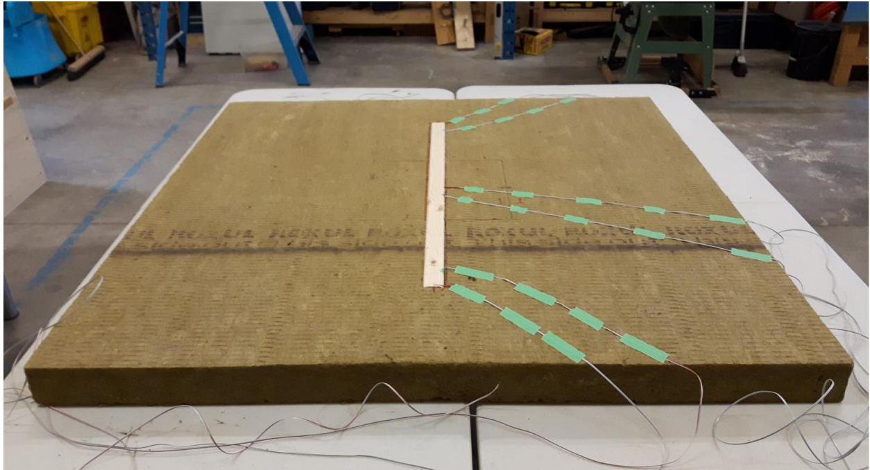
Wood stud installed in the first insulation sample used in the validation testing.
