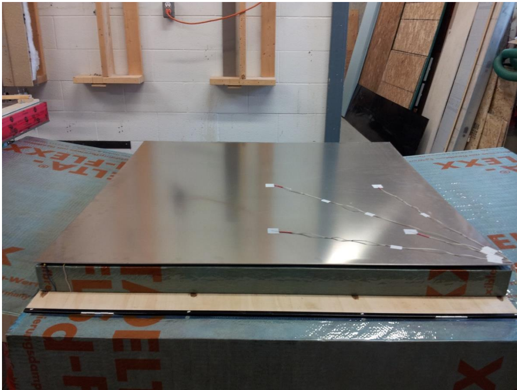
Back guard and back insulation installed on the apparatus frame. The hot plate assembly is not glued together or adhered to the frame.
