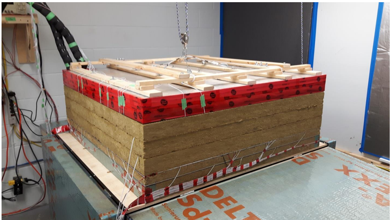
The 9" (229mm) specimen used for validation testing with the cold plate on top.
