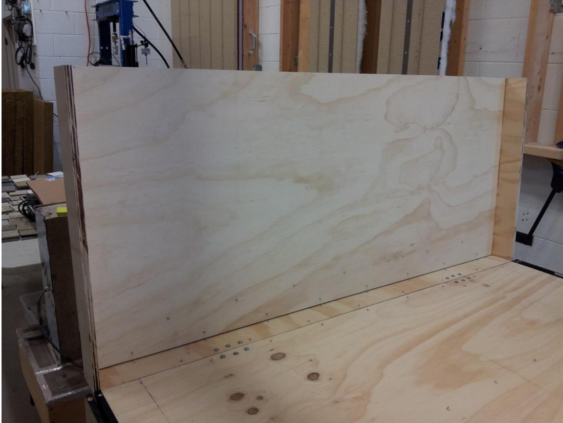
Side panel prior to edge insulation installation.
