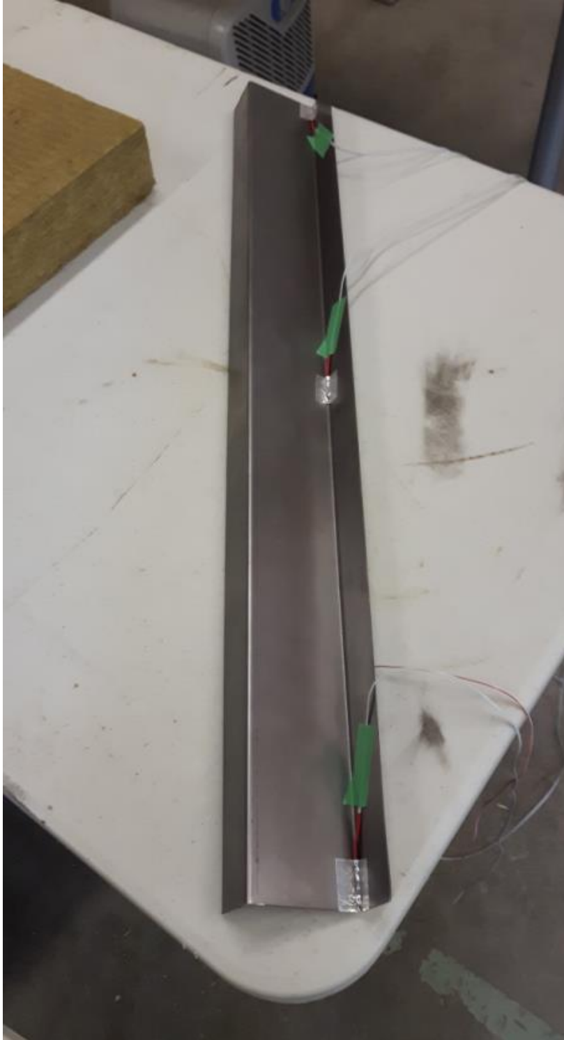
Steel Z-girt used in the thermal bridge testing. Thermistors are attached to the Z-girt in a similar pattern as the wood stud.
