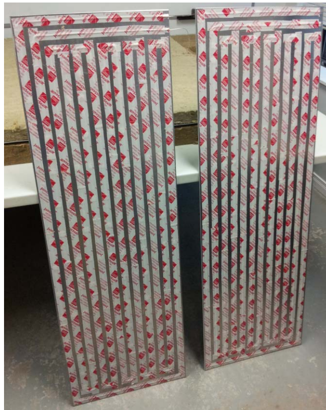
Figure 12 – Taped heater wire on the back of the top and bottom guard.
