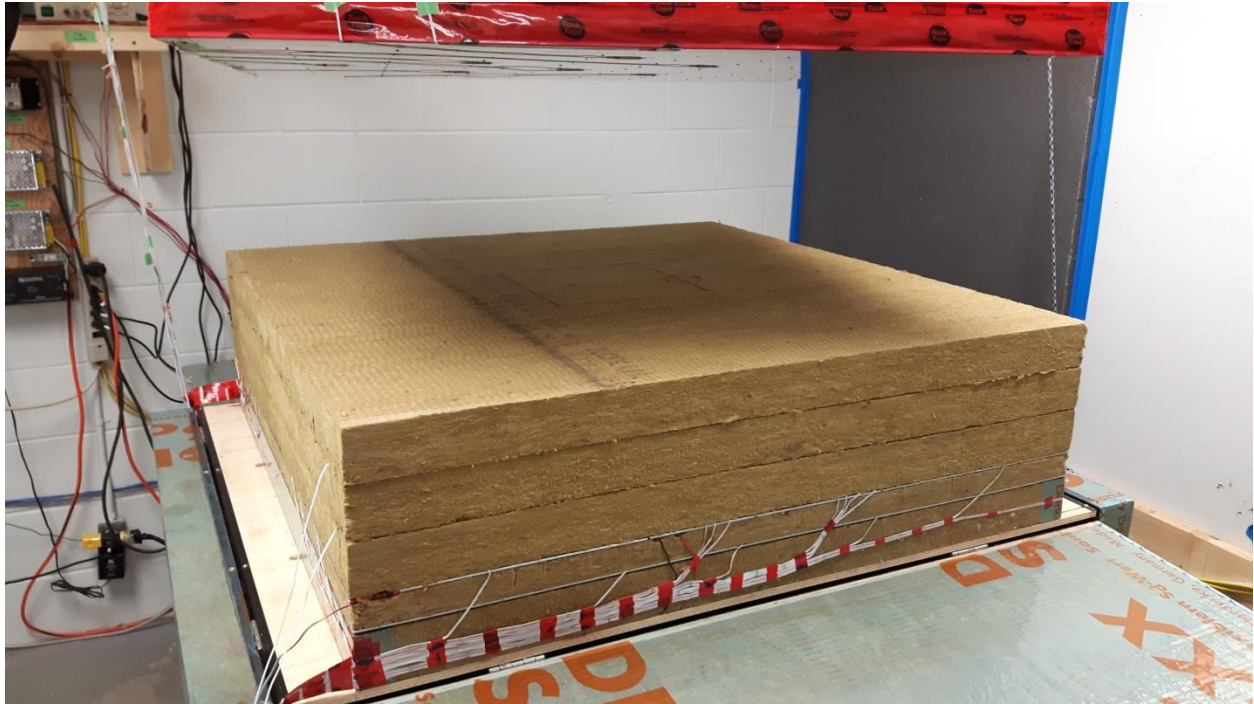
The 9" (229mm) specimen used for validation testing.
