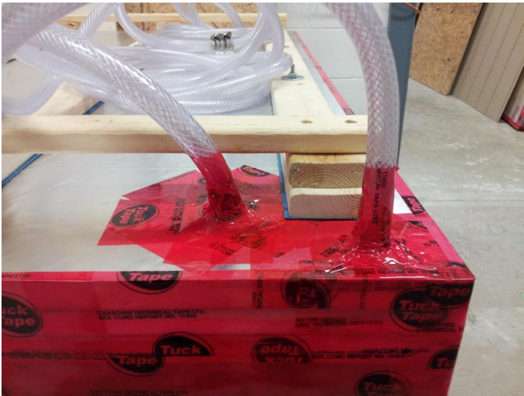
The inlet and outlet tubes coming out of the cold plate assembly.
