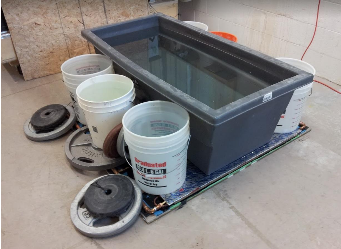
Weight applied over the cold plate and copper tubing during the curing of the thermally conductive epoxy.
