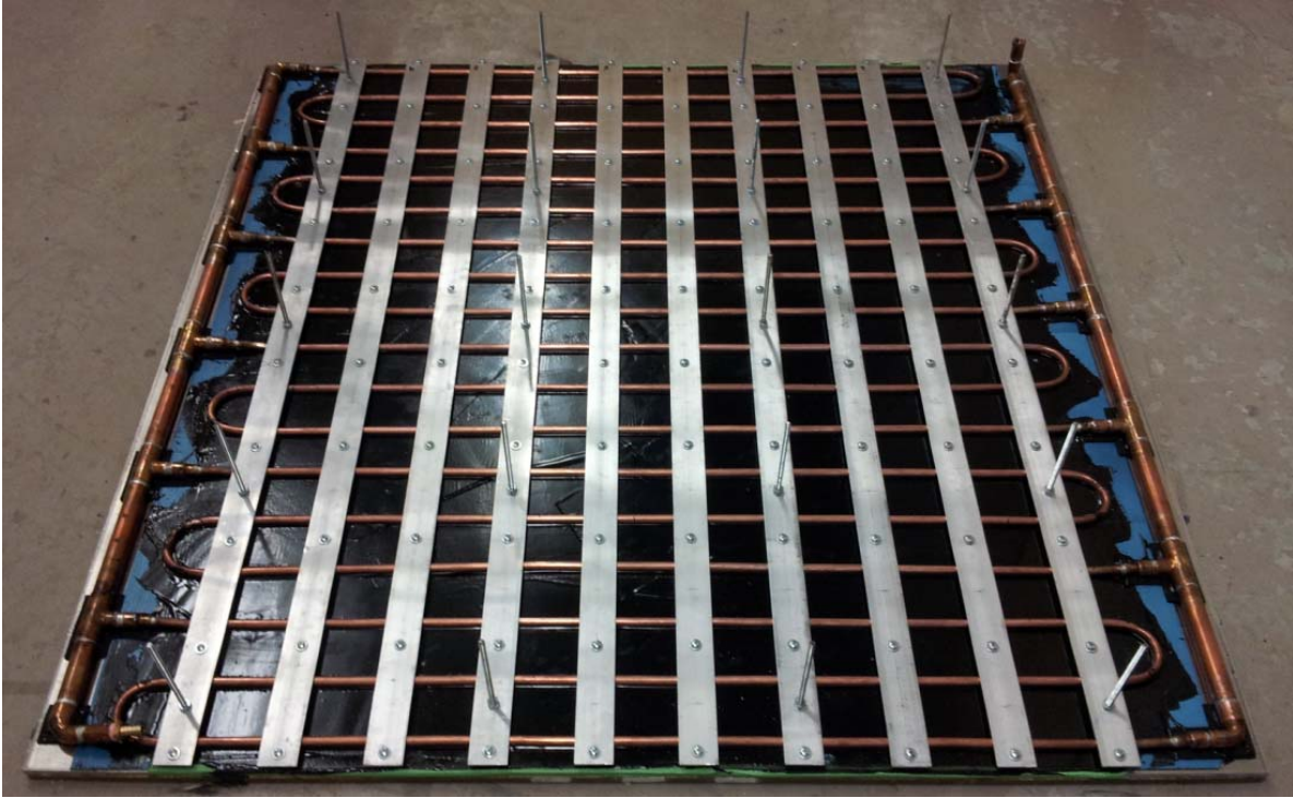
Figure 22 – Bar stock screwed in place clamping the copper tubing to the plate.
