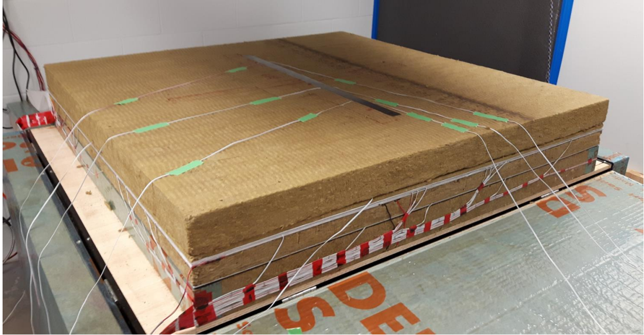
Steel Z-girt and insulation in the specimen stack.
