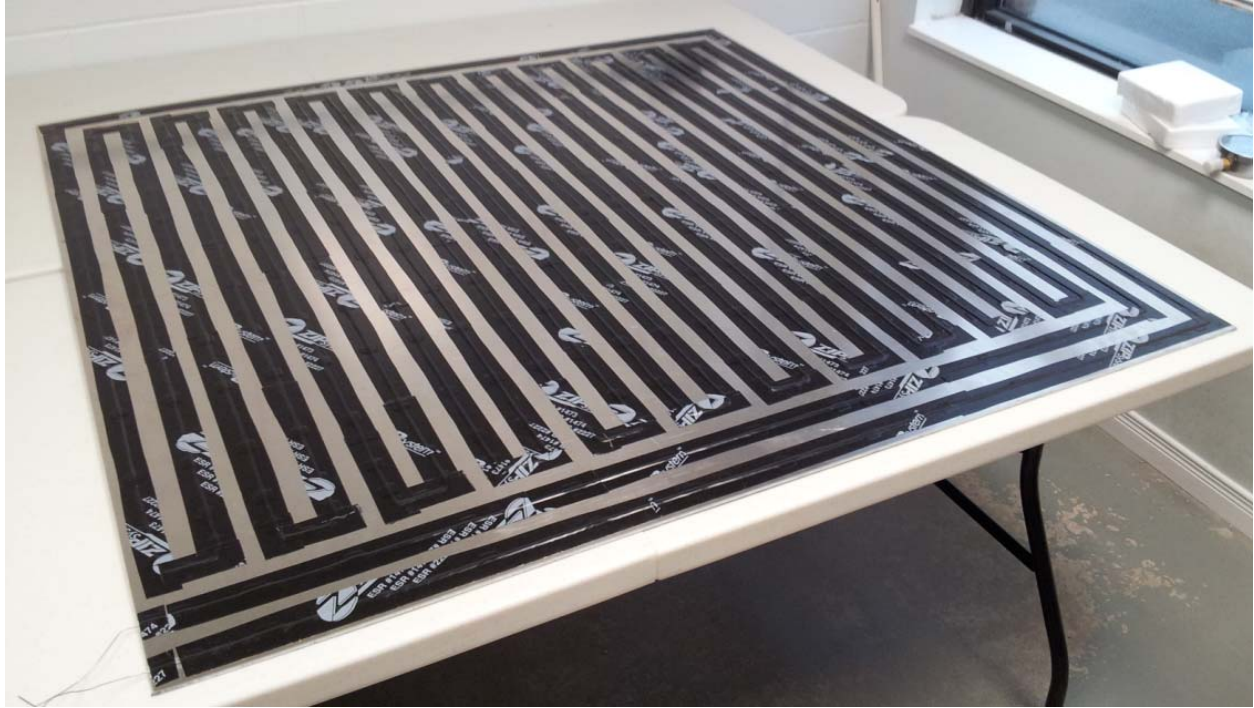
Figure 15 – Taped heater wire on the back guard plate.
