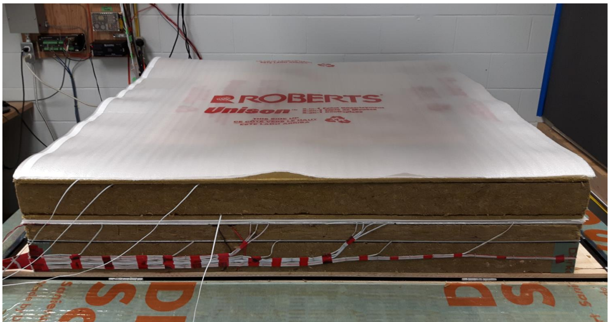
Top layers of foam representing a surface film in the thermal bridge testing.
