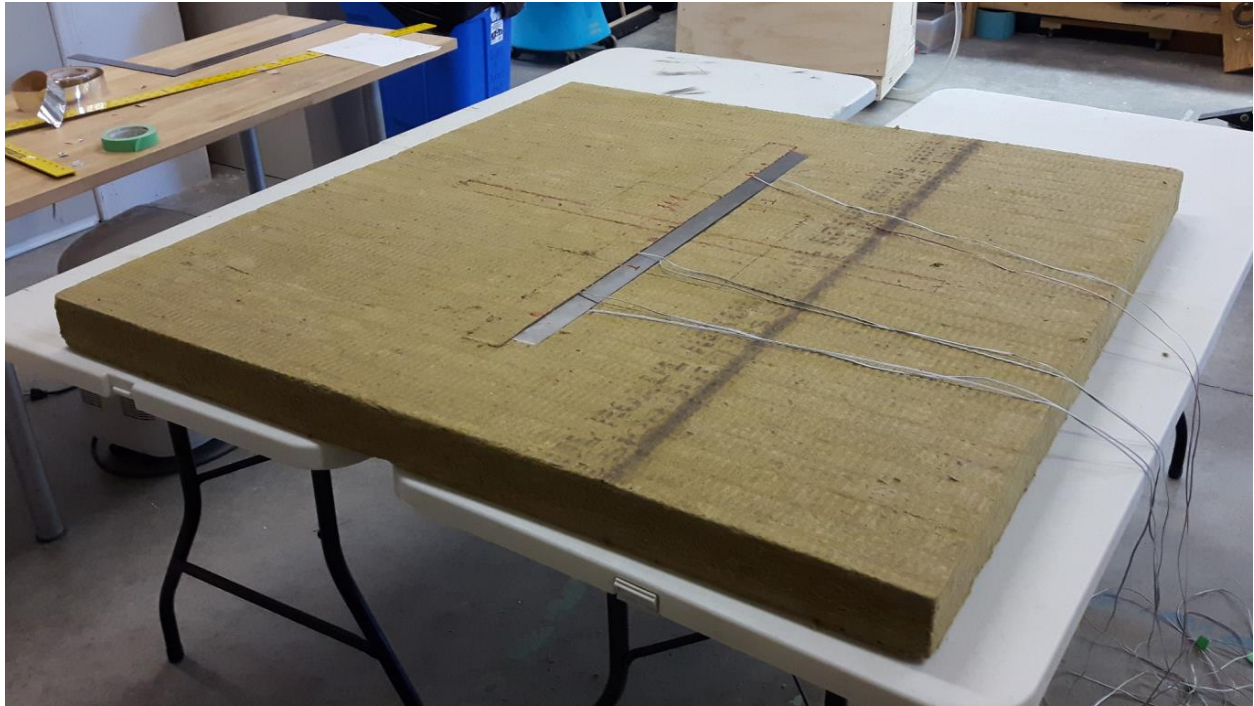
Steel Z-girt installed in the first insulation sample from the validation testing.
