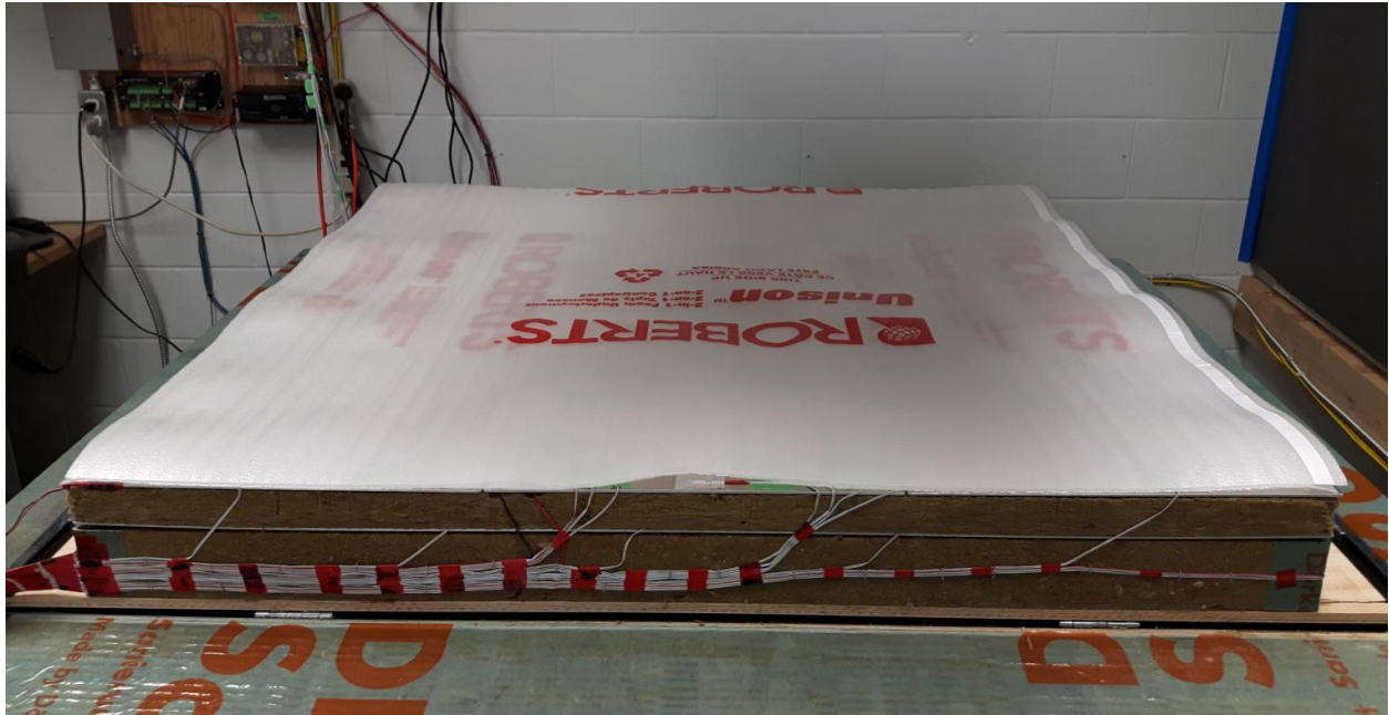
Bottom layers of foam representing a surface film in the thermal bridge testing.
