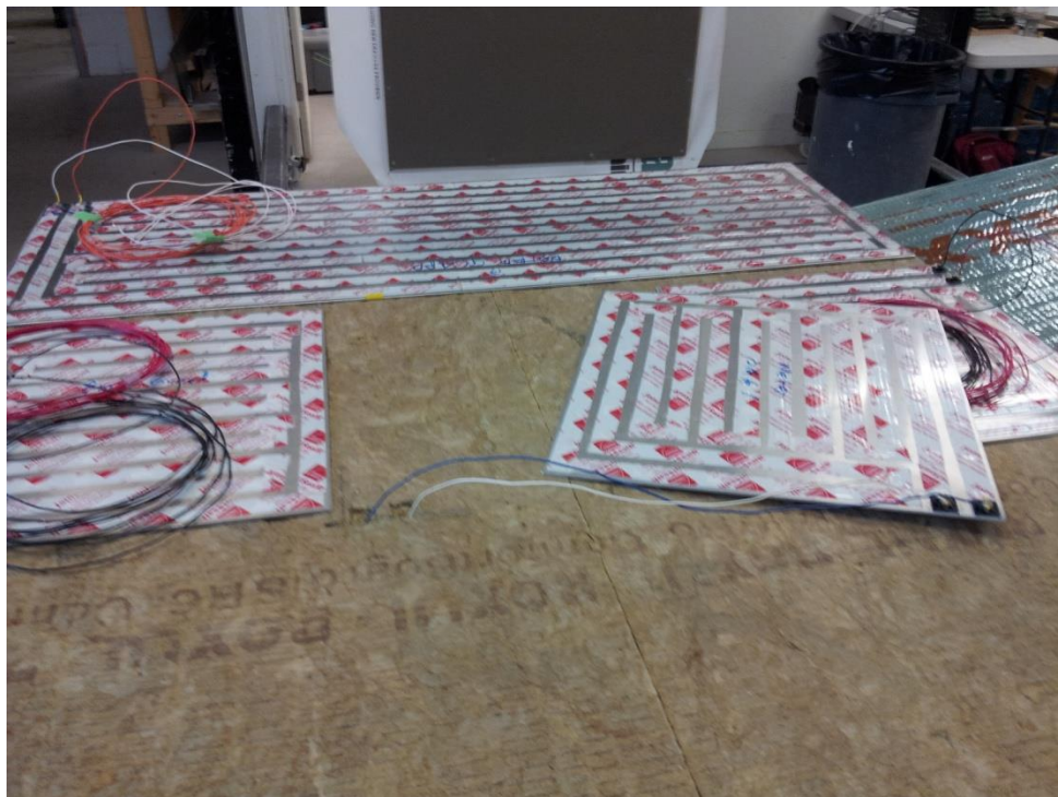
Meter plate and other guards being installed (shown upside down to show heater wire pattern).
