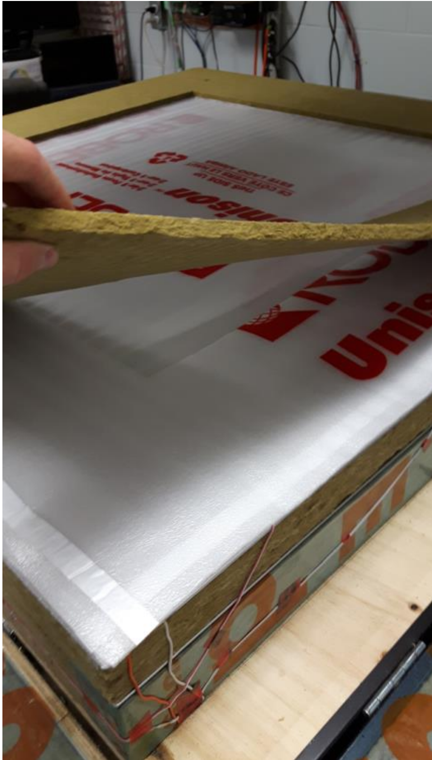
Detailed view of the Roxul Monoboard® layer and foam layers beneath.
