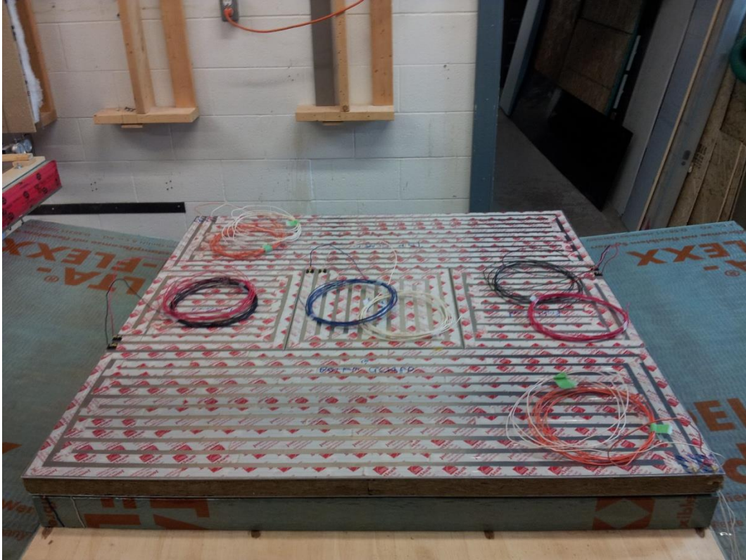
Meter plate and the top, bottom, left, and right guards upside down to show the heater wire pattern.
