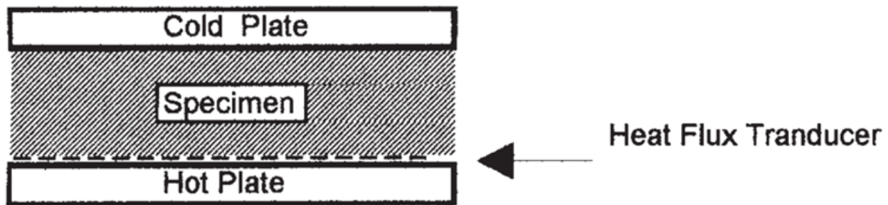
Figure 1 – Schematic of the heat flow meter (ASTM International, 2015).
