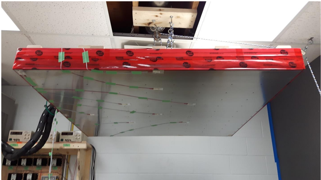
Thermistors on the cold plate assembly.
