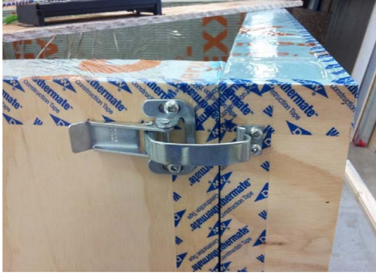
Figure 38 – Clamps used to hold the edge insulation panels in the closed position.
