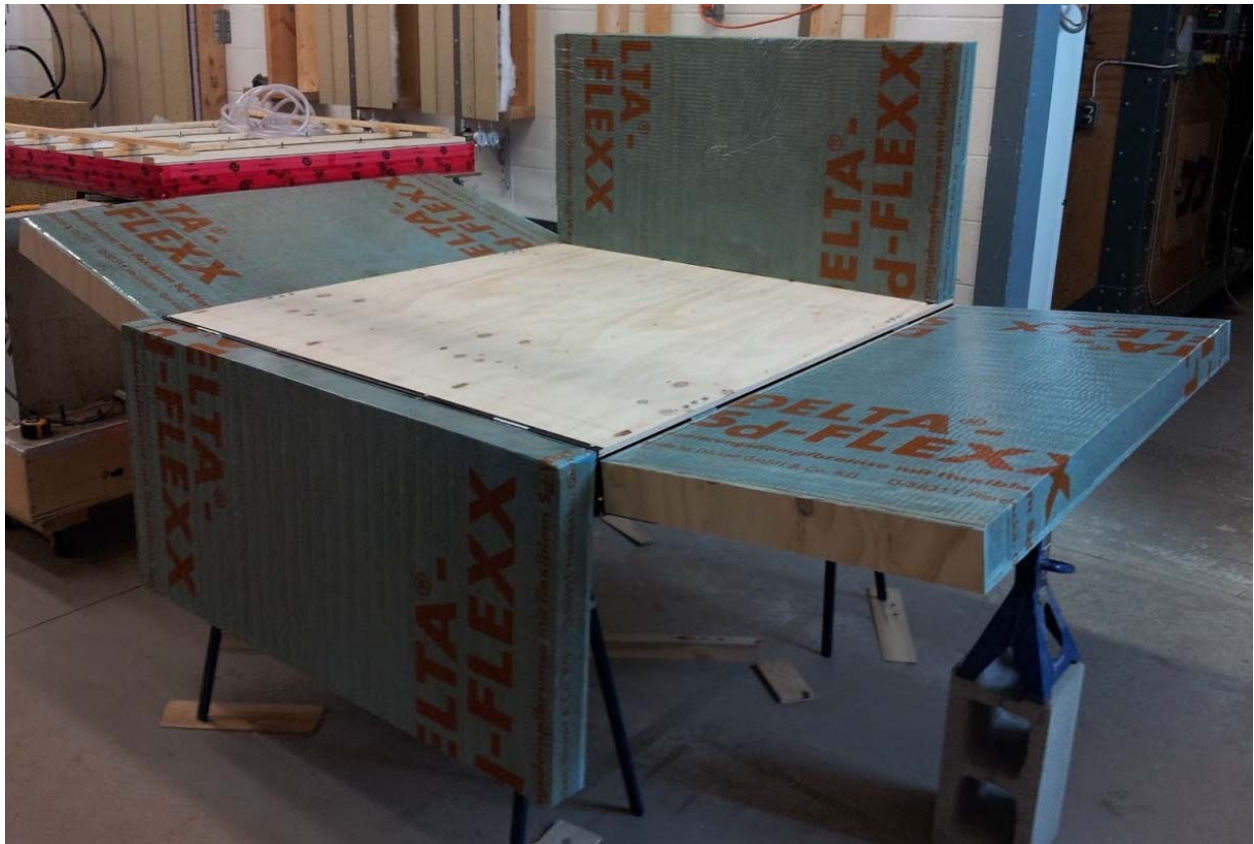
Figure 36 – Completed apparatus frame on temporary stands with edge insulation panels in the open position.
