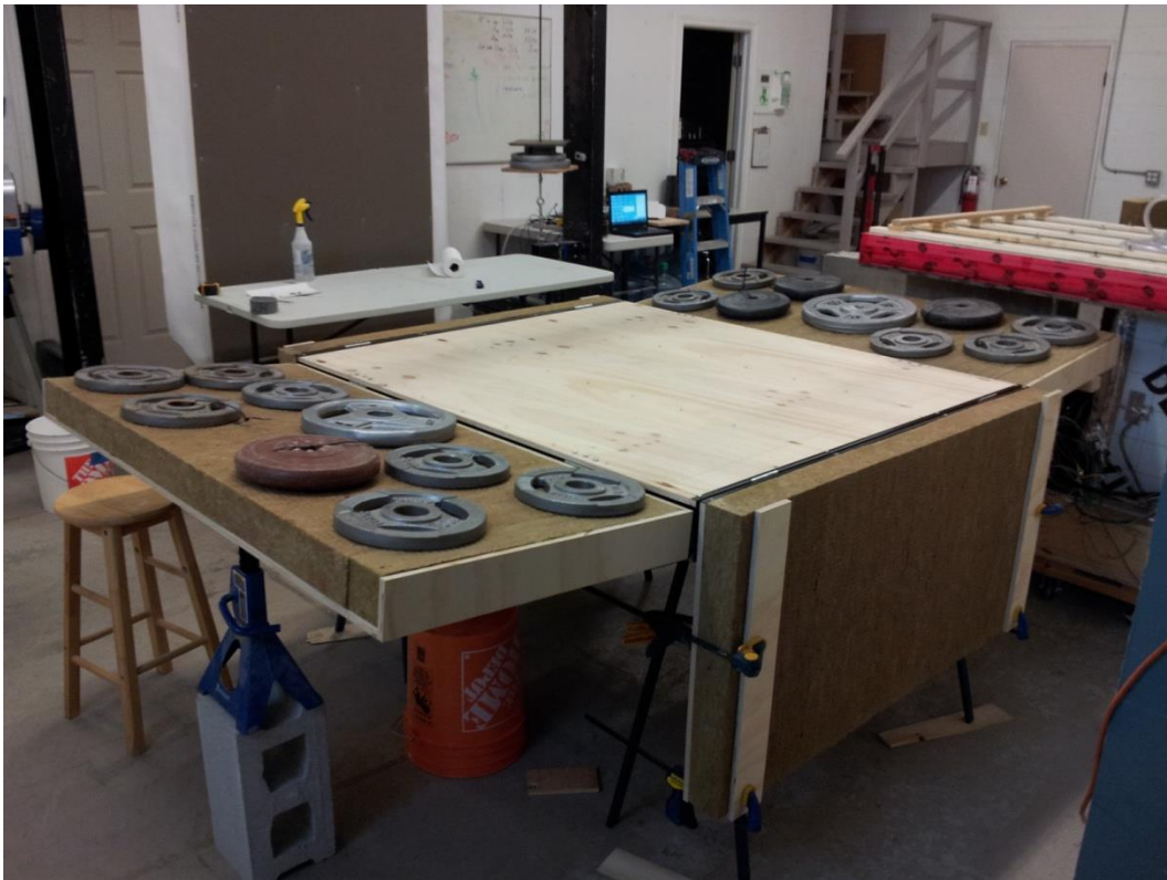
Installation of the edge insulation.
