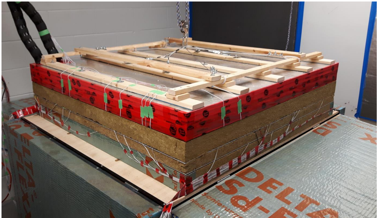
The 3" (76mm) specimen used for validation testing with the cold plate on top.
