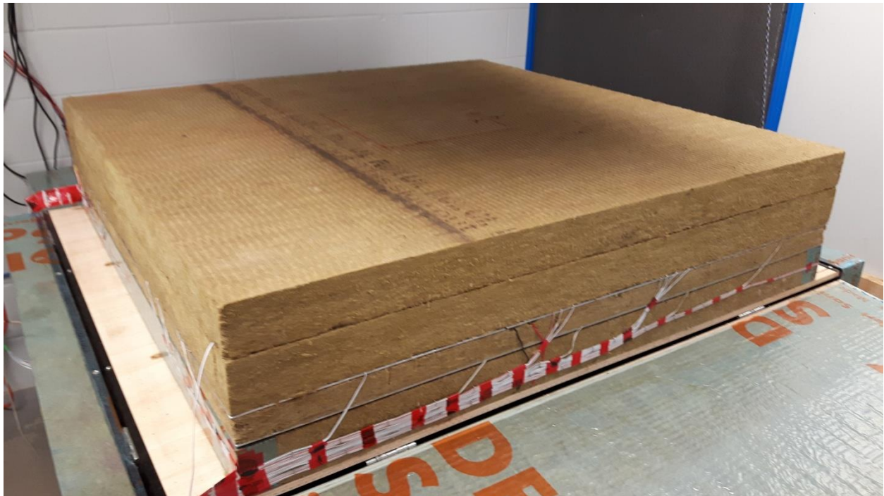
The 6" (152mm) specimen used for validation testing.
