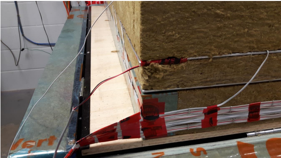
Bi-metallic switch installed in the hot plate assembly that opens if the assembly gets too hot unexpectedly.
