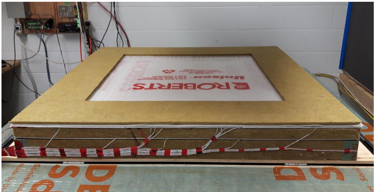
Roxul Monoboard® layer acting as a guard around the inner gypsum board layer (not yet installed).
