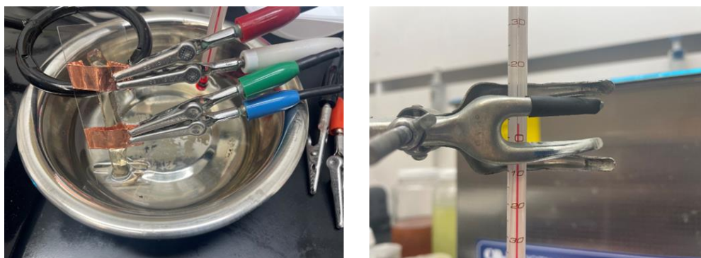
Figure 2.1 The experimental setup of ionic conductivity measurements.
