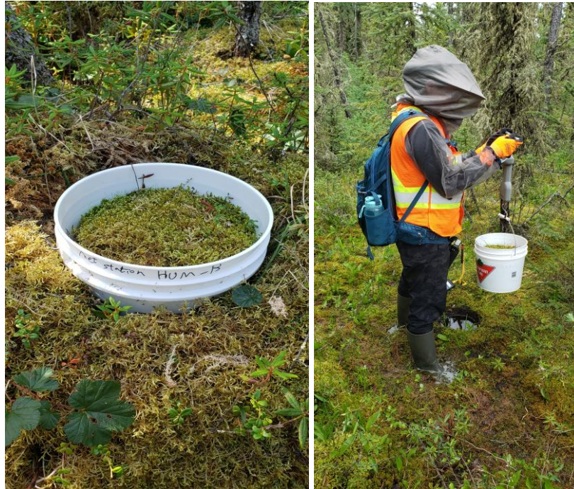
Figure 4-2 The weighing lysimeters to measure the actual evapotranspiration.
