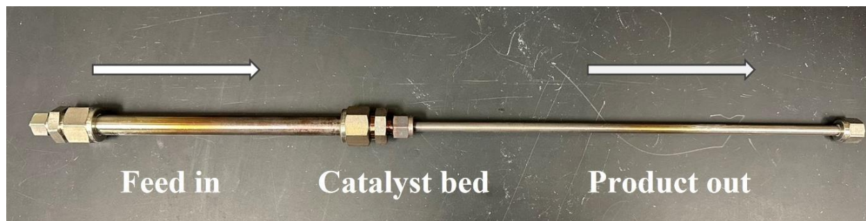
Figure S4. Kinetic reactor configuration.
