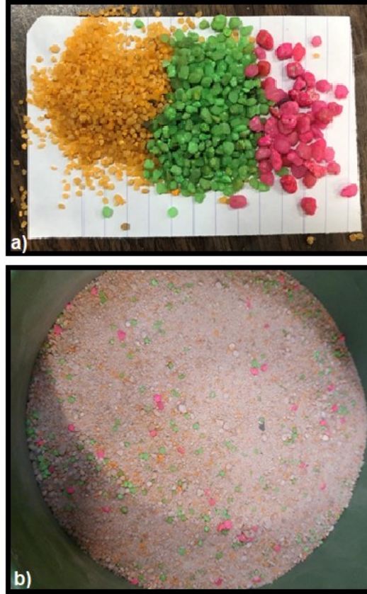
Figure 4.4 a) The three sizes of painted tracers used for this study under regular light. b) The final sediment mixture used for the current study under regular light
