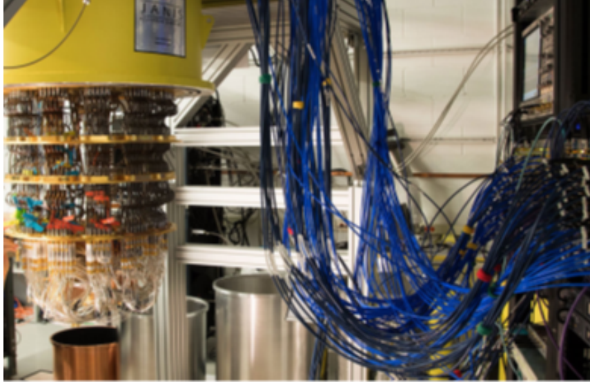
Figure 1.1: Google’s Sycamore processor. Blue coaxial cables are connected from custom analog control electronics (on the right) to the quantum processor. Source: [5]
