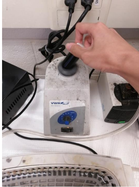
Figure 58: Vortexer for dry powder mixing
