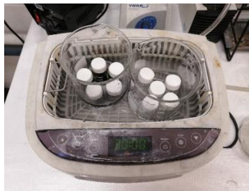
Figure 16: Bath Sonicator with 10 sample vials
