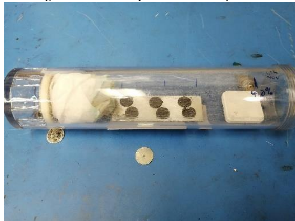
Figure 36: Humidity Chamber Interior with 6 sensors
