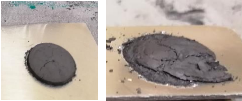
Figure 28: Non-plasma treated CNF (Left) Vs. Plasma Treated CNF (Right)
