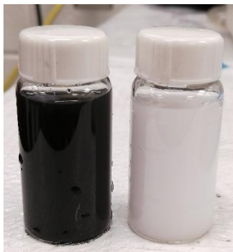
Figure 17: Carbon Nanotube Dispersion (Left) & TiO 2 Dispersion (Right)
