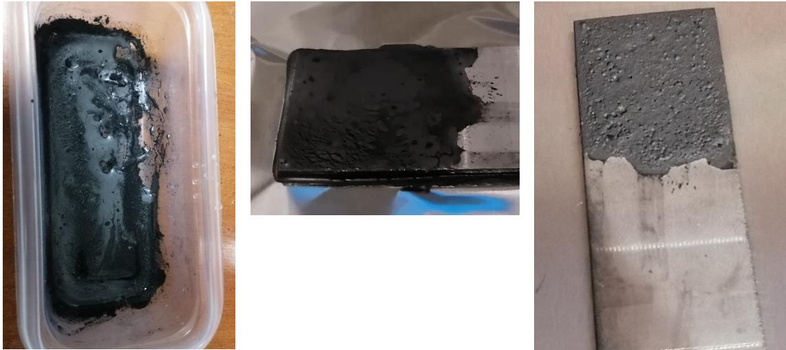
Figure 22: IPA Suspension (Left), Magnesium Coating (Mid), Post-baked (Right)
