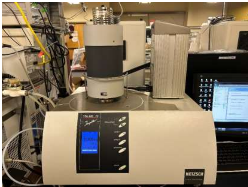
Figure 2.4 The NETZSCH STA 449 F3 Jupiter DSC machine used for this thesis
