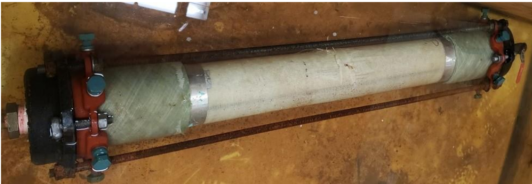
Figure 3.7: A 150mm OD CIPP Pressure Liner specimen, prepared and used in a short-term burst test (Source: Awe, 2023)
