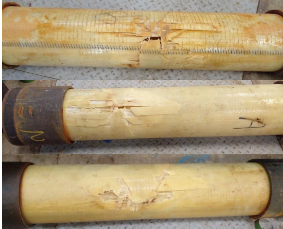
Figure 3.20: Failed CIPP Pressure Liners during Short-term Tests
