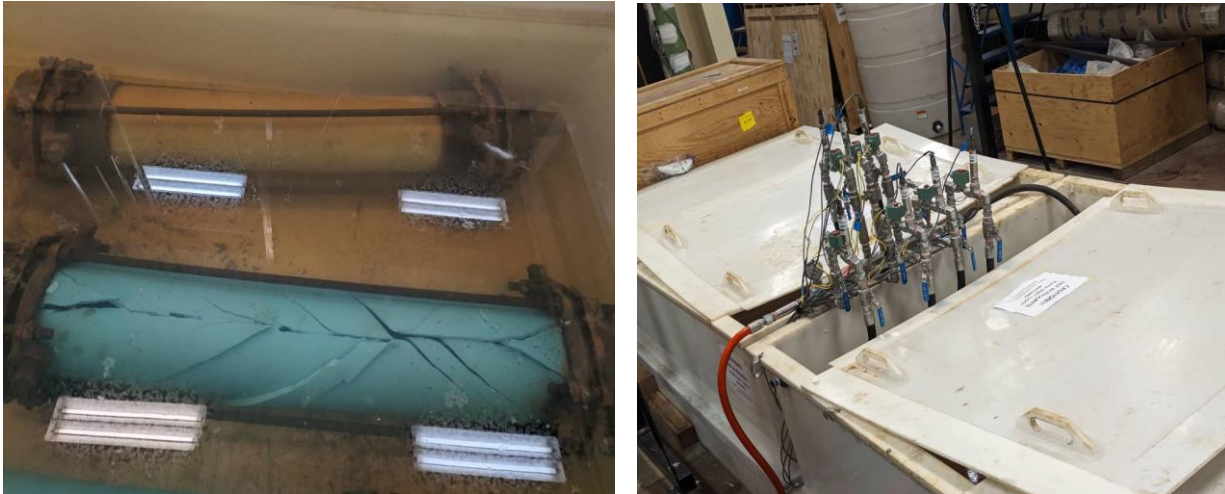
Figure 3.5: Plastic water tanks and submerged test specimens
