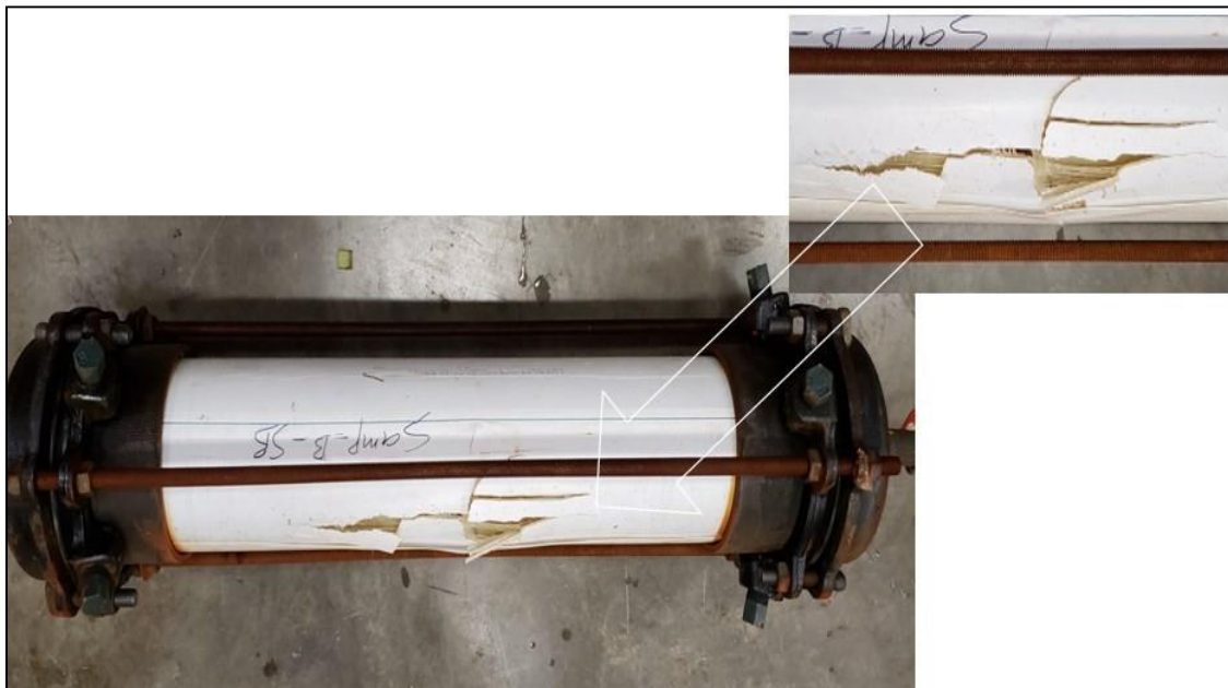
Figure 3.11: Sample of CIPP specimens' middle failure in a short-term burst test (Source: Awe, 2023)
