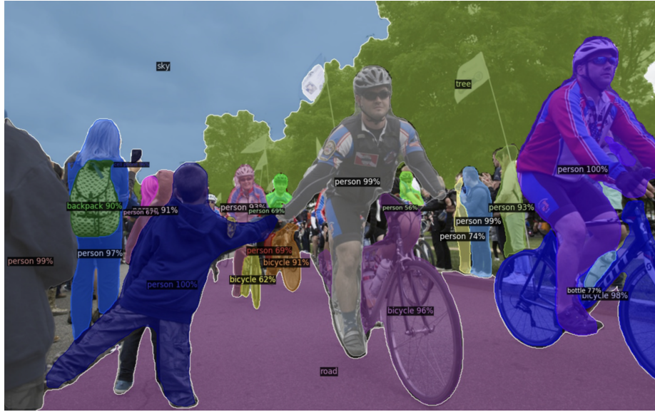
Figure 3.13: An image processed using Detectron2’s Mask-RCNN model demonstrating its ability to segment and classify multiple objects in an image [57].
