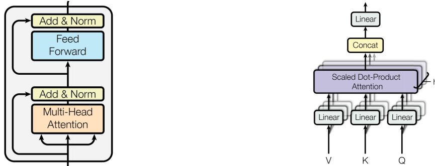
Figure 2.1: The model structure of a transformer layer (left) and the multi-head attention mechanism (right). 9
