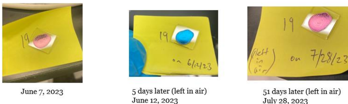
Figure 2-6: Time-lapsed photos showing that the DPPPy-TT doped with 10mol% FeCl 3 , which was not successfully doped, shows a dramatic color change around 5 days later which eventually fades away.
