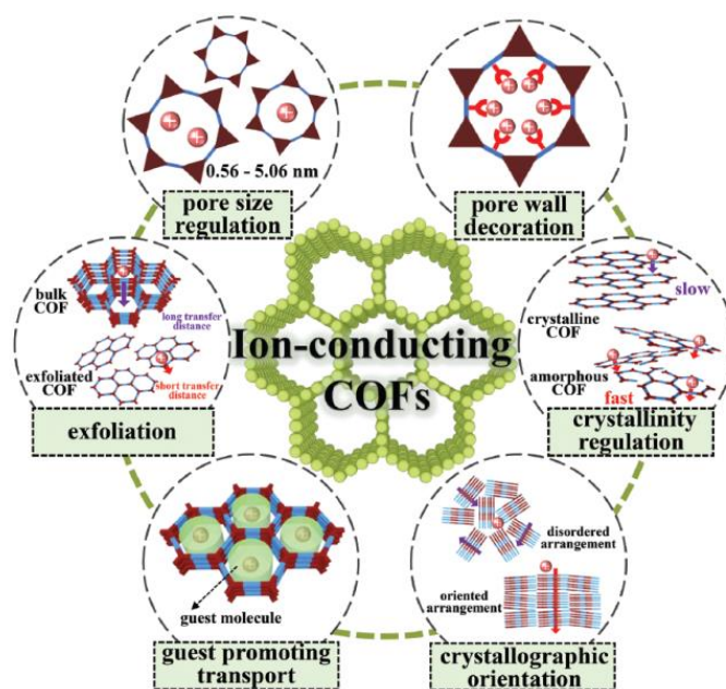
Figure 1.13 Schematics of strategies for ion-conducting COF design. 87 Reproduced with permission from Ref. 87, copyright 2022. Wiley-VCH GmbH.
