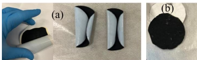
Figure 3.7 Photographs of (a) modified PP separators and (b) modified GF separators at 50°C in a vacuum oven.
