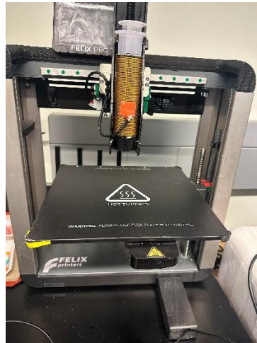
Figure 11: Syringe-based 3D Printer used in the 3D Printing of CSBP. FelixFood Single Head 3D Printer.
