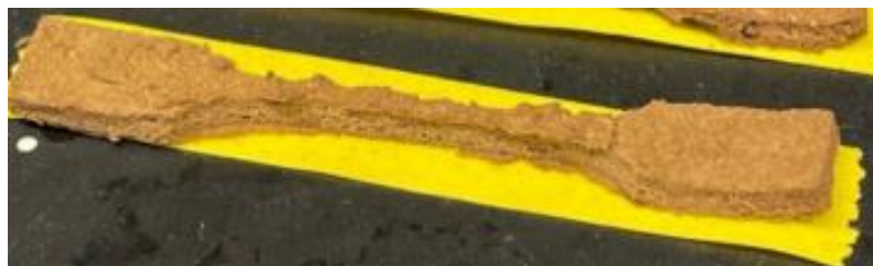
Figure 10: 3D Printed Heat Cured CSBP Dogbone. Samples was 3D printed and heat cured at 200°C for 30 minutes.
