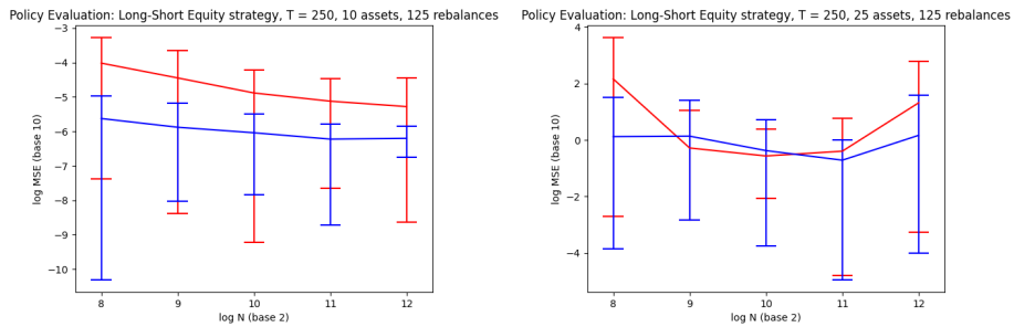
Figure 9: For each plot MC is graphed in red and RQMC is graphed in blue. The upper bounds represent the maximum squared error from the 30 random experiments, the lower bounds represent the minimum squared error, and the trend line shows the MSE. For this choice of reward function we see very poor policy evaluation performance for the 25-asset case.
