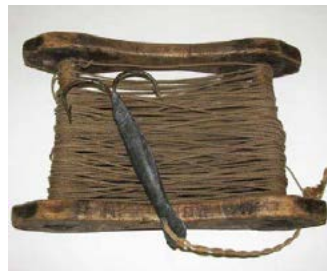
Fig 3.24 Cod Jigging Reel. This old fashioned technology remains as a sustainable method of fishing.
