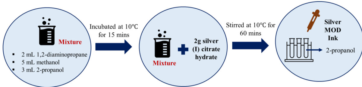
Figure 20: A schematic of the Ag MOD ink formulation procedures
