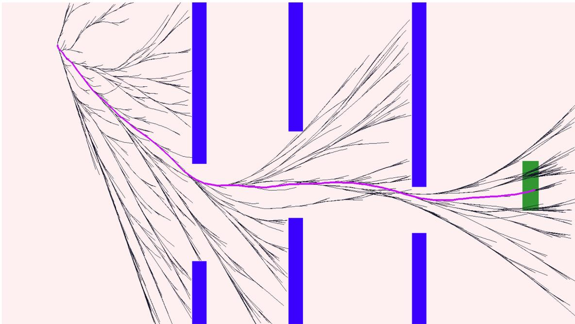
Figure 2.3: An example of a tree produced by  $SST$  for the flappy bird problem. The initial state is in the top-left, the point travels at a constant horizontal velocity, and the control-space is a set containing only two options: “do nothing”, or “accelerate up”, each for a random duration. The least-cost solution for this execution is highlighted in pink.
