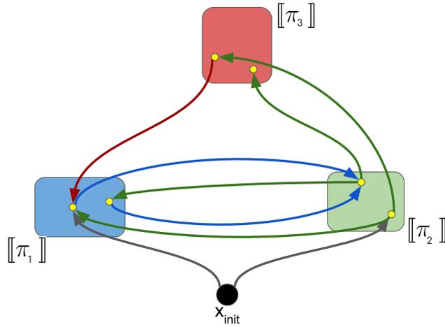
Figure 4.8: This diagram illustrates the set of solution trajectories found when attempting to reach from every sampled node of each proposition region (and initial state  $x_{init}$ ) to all other proposition regions. We use  $m = 2$  samples in this example.
