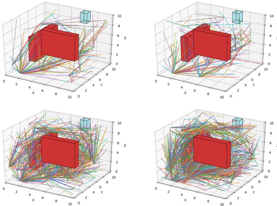
Figure 4.2: Shown here are the tree structures generated for four different configurations. Starting from the top-left and reading across, we list the pairs  $(N_p, J_{th})$  used:  $(200, 300)$ ,  $(200, 260)$ ,  $(1000, 200)$ ,  $(2000, 150)$ . Edges represent collision-free paths between pairs of waypoints. Note that the visualization software displays an unobstructed view of at least one object, giving the false impression that no edges exist in front of the clearly visible obstacle.
