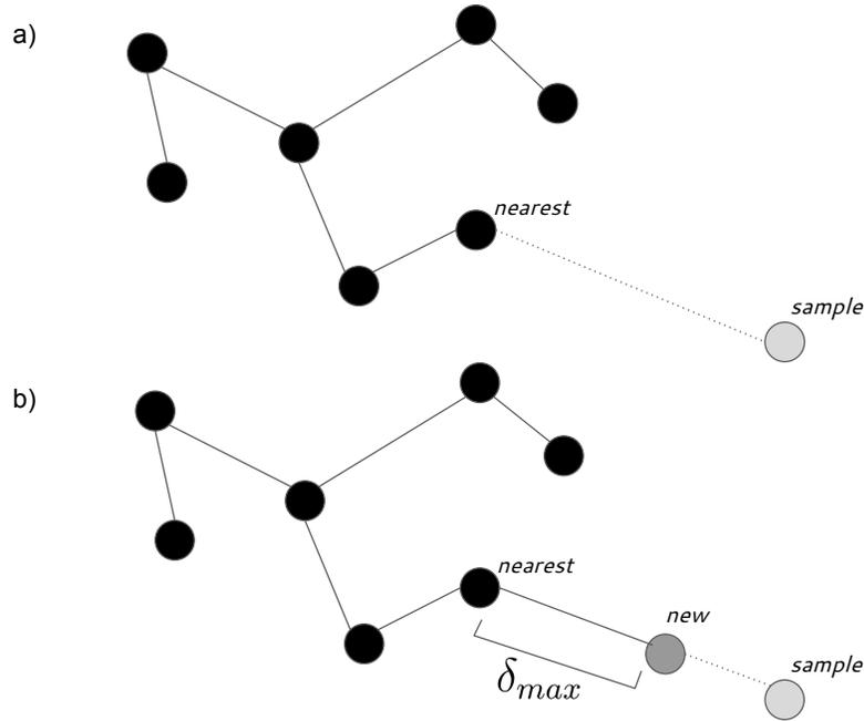
Figure 1.1: [RRT](#) sampling and connection procedure. The existing tree is shown with black nodes and solid edges. a) A node is randomly sampled from the state space, and the nearest existing node is found. b) A new node and edge are added to the tree along the line connecting the nearest and sampled nodes, but at a maximum distance  $\delta_{max}$  from the nearest node.
