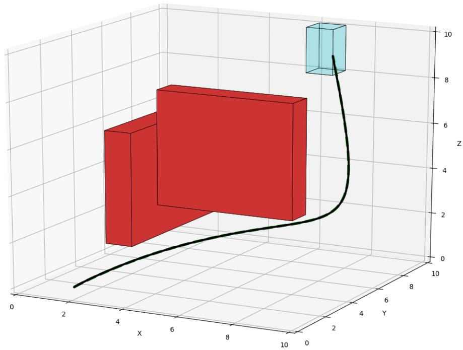
Figure 4.7: Tracking the polynomial trajectory generated for the  $N_p = 200$ ,  $J_{th} = 260$  configuration (top-right instance of [Figure 4.4](#)). The nominal trajectory is shown as a dashed green line, though it is obscured by the simulated trajectory obtained using the tracking controller (black).
