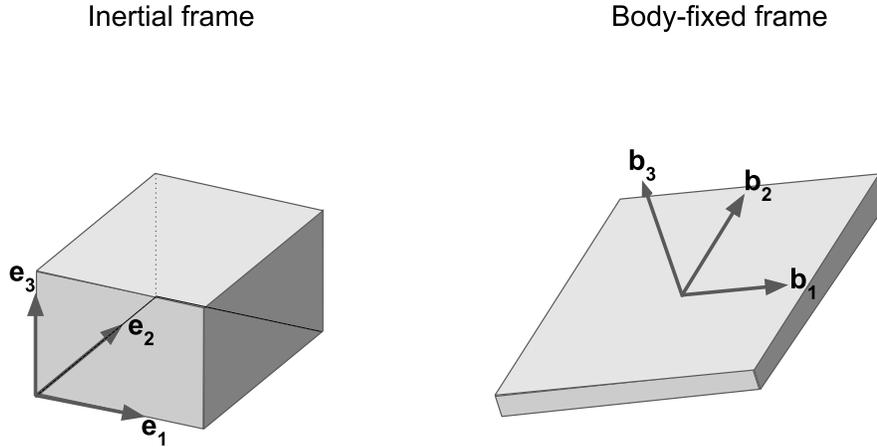
Figure 4.1: The inertial frame and the body-fixed frame are shown, where the origin of the body-fixed frame is placed at the centre of mass of the quadrotor, which is represented as a flattened rectangular prism.
