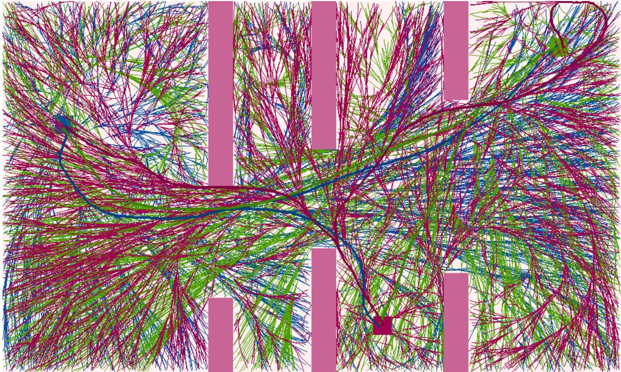
Figure 3.2:  $SST^*$  is performed three times, producing a Kripke structure for each of the regions shown here in blue (left), burgundy (bottom center), and green (top right). Obstacles are represented as pink rectangles. The color of each line matches the color of the region of the Kripke structure to which it belongs, and the bolded curves are the lowest-cost trajectories that reach another region.
