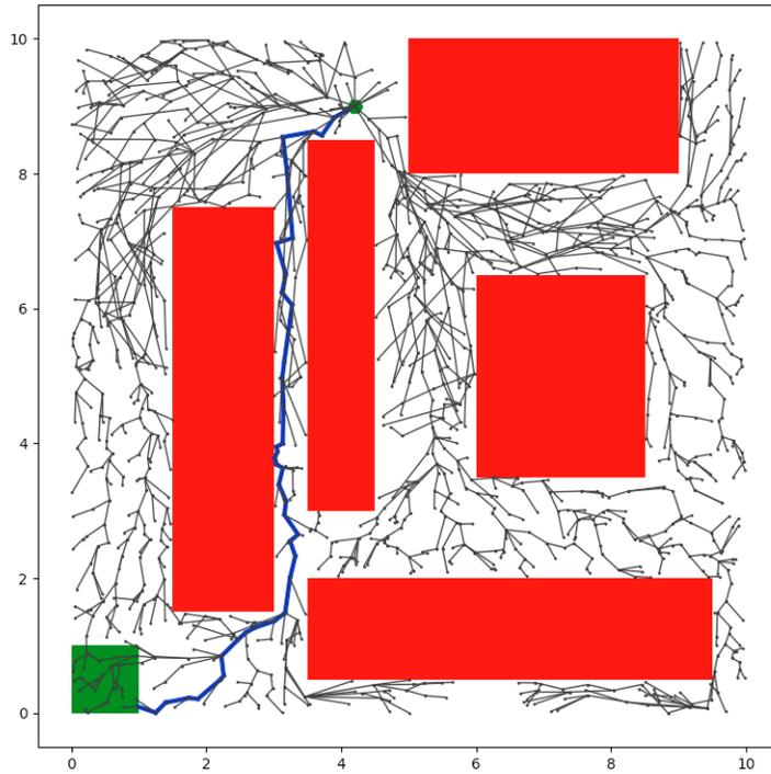
Figure 2.4: Example of a tree generated by  $\text{FMT}^*$  using 2000 nodes. The initial state is shown at the top center as a green hexagon, the goal region lies in the bottom left and is shown in green, and obstacles are represented by red rectangles. The optimal path is highlighted in blue. This example does not use any dynamic model, so the cost function is simply the Euclidean distance.
