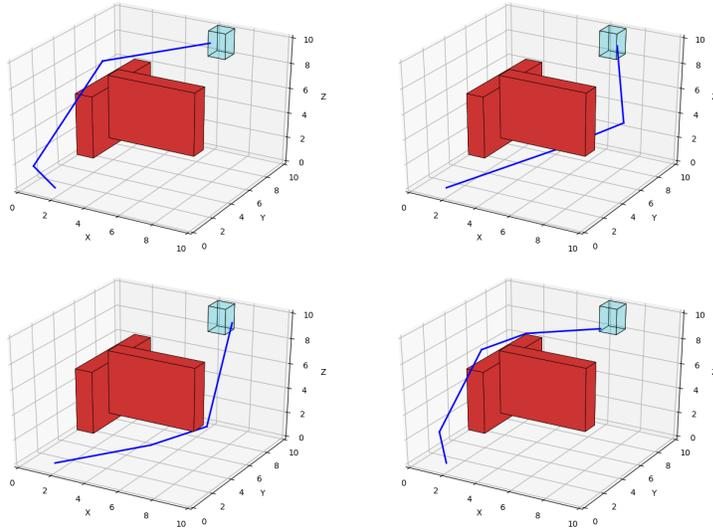
Figure 4.3: Here we see the best-path waypoints as seen before smoothing is applied. `kinoFMT` returns a piecewise-linear path connecting the waypoints returned, shown in blue. The four configurations appear in the same order as in [Figure 4.2](#).
