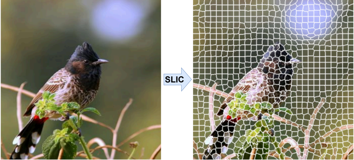
Figure 1.1: Visualization of Superpixels. An example of superpixel segmentation. (Left) Original input image. (Right) Superpixel representation, where pixels are grouped into compact, perceptually similar regions. This representation reduces spatial complexity while maintaining important object boundary information.
