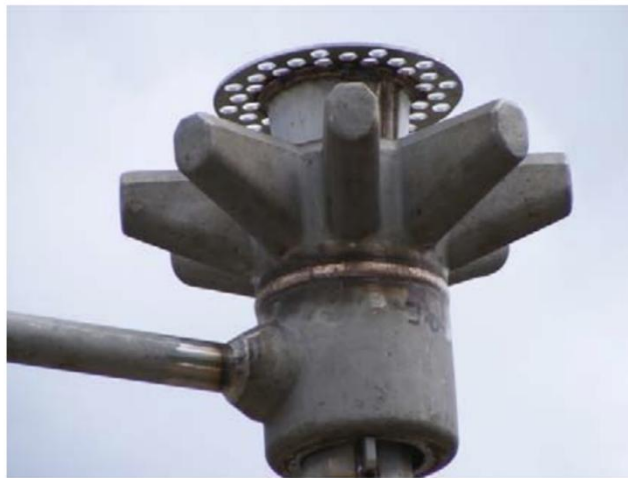
Figure 4.8 John Zink SKEC ® flare tip. Adapted from Ref. [97].
