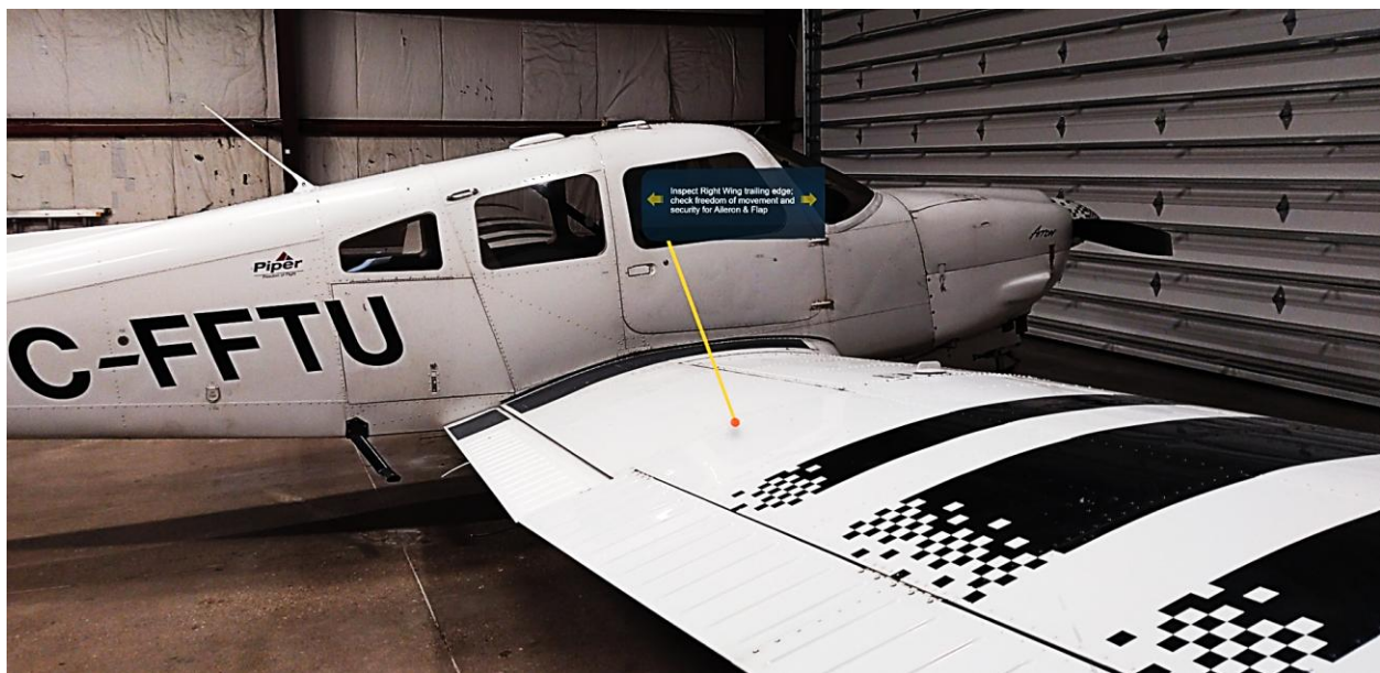
Figure 29 . AR instructional overlay shown in participant's field of view, assisting right-wing inspection.
