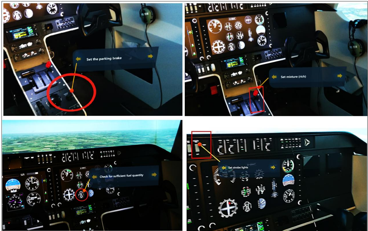
Figure 17. Examples of AR cues presented during the training simulation of P1 using M2, guiding the participant through steps such as setting the parking brake (top left), adjusting the mixture (top right), checking fuel quantity (bottom left), and activating the strobe lights (bottom right)
