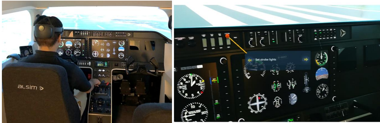
Figure 9: Student pilot using AR-integrated HMD in a flight simulator (left) and a snapshot from 'Before-Takeoff' checklist video showing a real-time AR instructional cue to set strobe lights (right)
