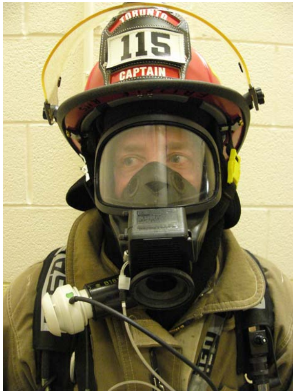
Figure 1: Front view of the modifications made to the MSA SCBA facemask to integrate the Cosmed K4b 2 system.
