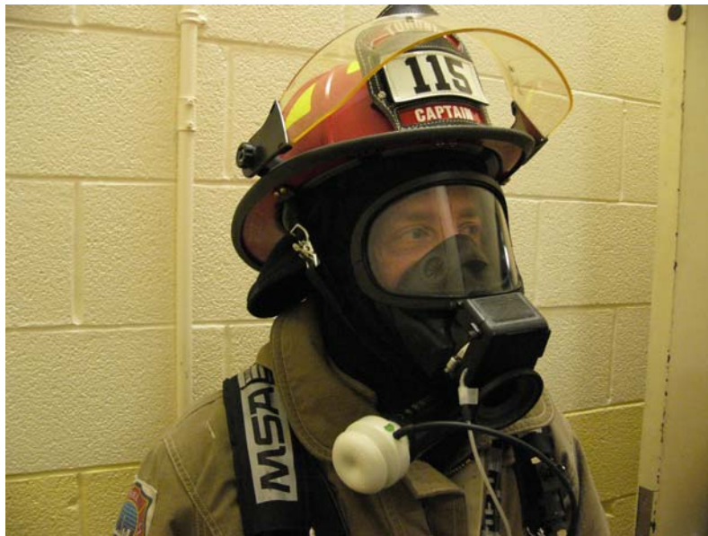
Figure 2: Side view of the modifications made to the MSA SCBA facemask to integrate the Cosmed K4b 2 system.
