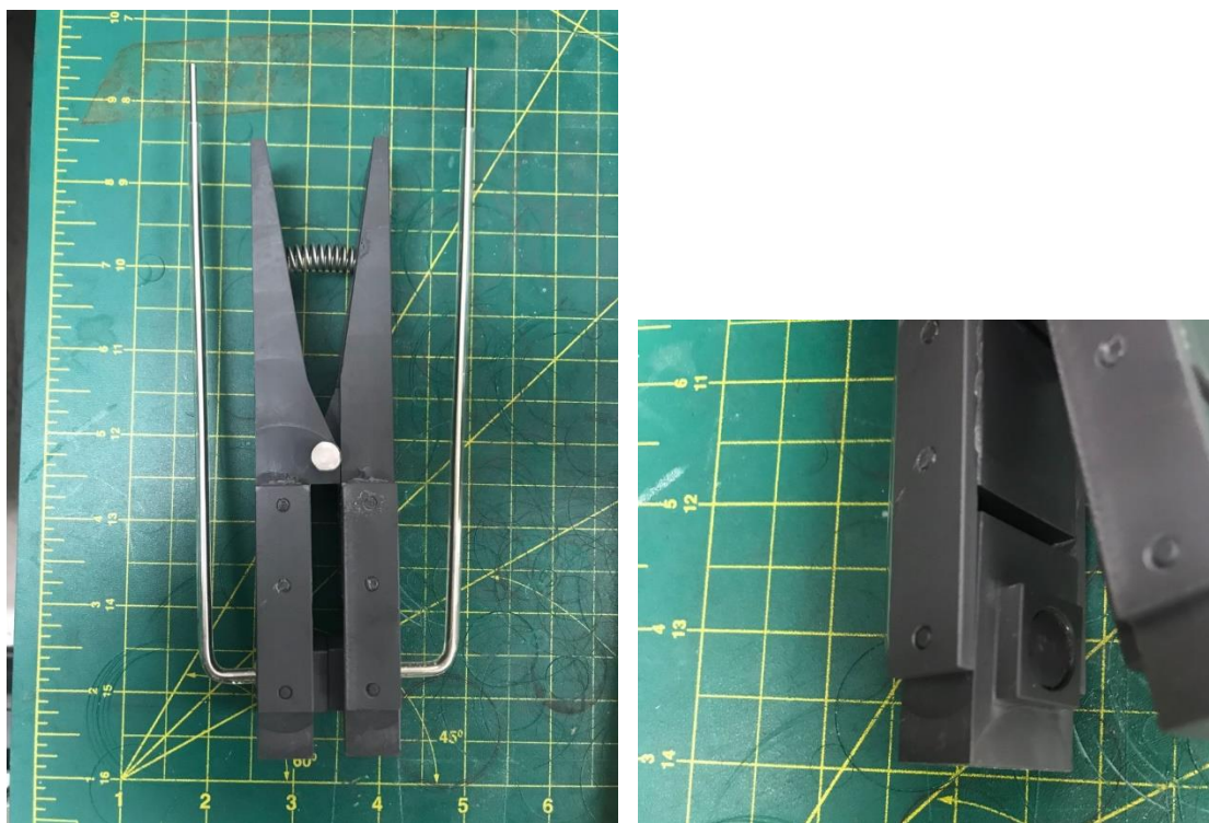
Figure 19: 2-electrode resistance clamp used for measurements
