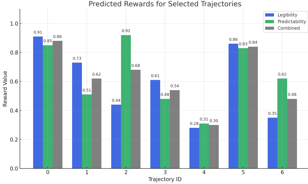
Figure 4.22: Predicted reward components for selected trajectories. High-performing behaviors (e.g., Trajectories 0, 5) exhibit both legibility and predictability, while ambiguous or erratic behaviors (e.g., Trajectory 4) score poorly across all criteria.
