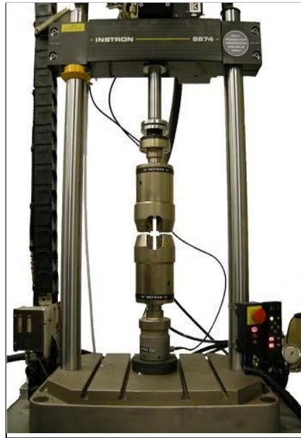
Figure 3:7: Instron 8874 machine. This machine is equipped with an axial force capacity of \pm 25 kN
