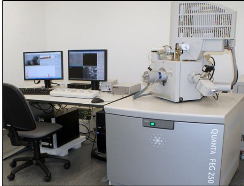
Figure 3:5: shows the scanning electron microscope (SEM). The LEO 1530 microscope and the FEI Quanta FEG 250 environmental scanning electron microscope (ESEM) were used, which was equipped with energy-dispersive X-ray spectroscopy (EDX) capabilities
