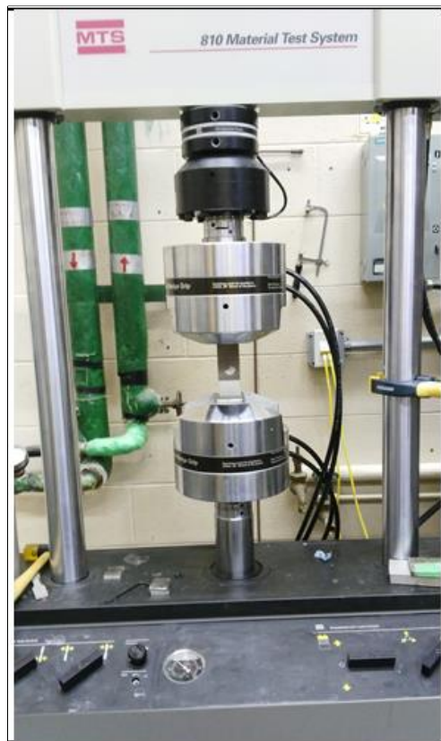
Figure 3:6: The MTS 810 material test system with a load capacity of up to 50 kN
