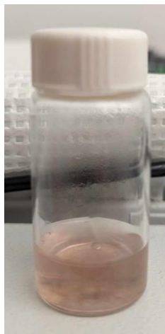
Figure 4.2. Image of gold nanorod hydrogel formulation using 3 % w/v hyaluronic acid. It forms a viscous, pinkish paste.
