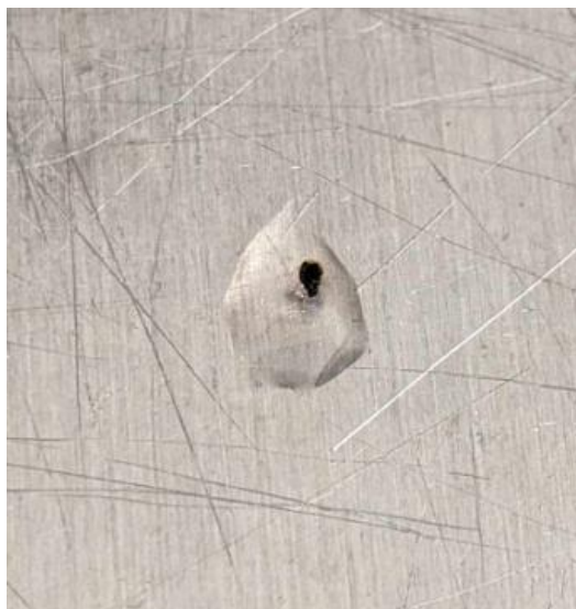
Figure 4.6. Image of 3 % w/v hyaluronic acid hydrogel on aluminum plate after laser irradiation at 7.8 W/cm 2 for 10 s. Carbonized material (black speck) appears on the surface of the hydrogel.
