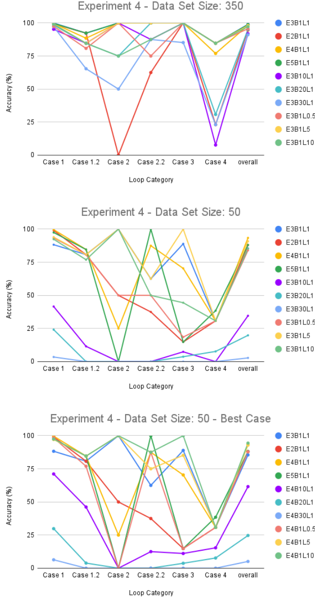
Figure 4.7: The charts illustrate the impact of different hyperparameters. Top: model fine-tuned with 350 instances. Center: 50 instances. Bottom: The best results are from the center chart. E: Number of Epochs, B: Batch Size, L: Learning Rate [2].
