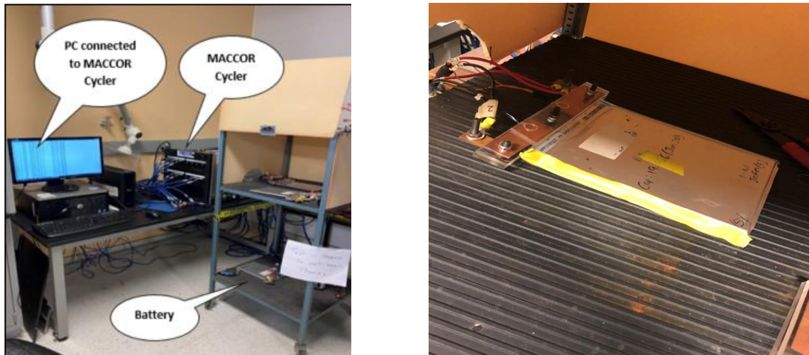
Figure 6.1: Experimental setup: experimental setup and MACCOR 4200 battery cycler (left); and tested 20Ah battery pouch cells (right).
