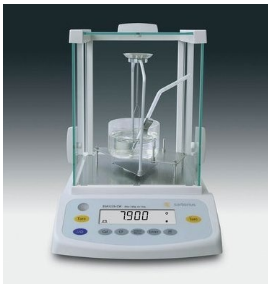
Figure 3.11 Custom setup for measuring the relative density using Archimedes' Principle
