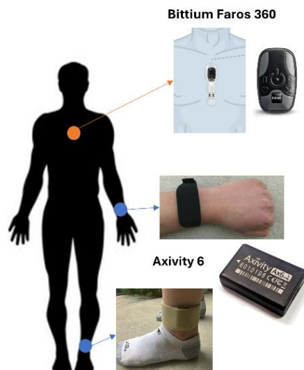
Figure 2. 1. Participant set up with devices. Schematic representation of wearable device type and location on body segments, including Bittium Faros 360 device on chest and Axivity 6 devices on wrist and ankle.
