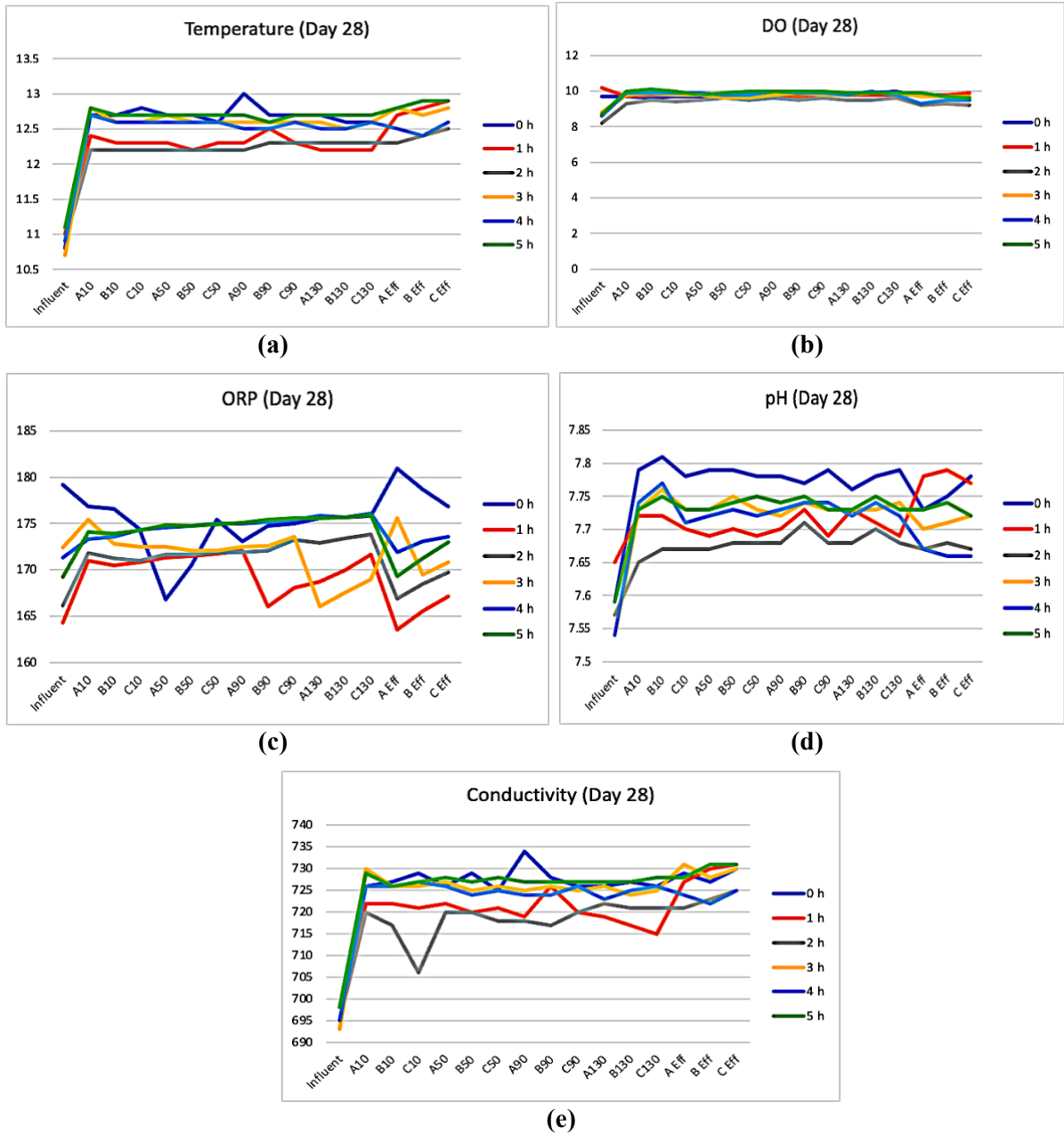
Figure B.3 Impact of 18-h shutdown on water quality parameters during biofilter C start-up, on day 28 of operation (a) Temperature (°C) (b) pH (c) DO (mg/L), (d) ORP (mV), (e) conductivity (μS/cm)
