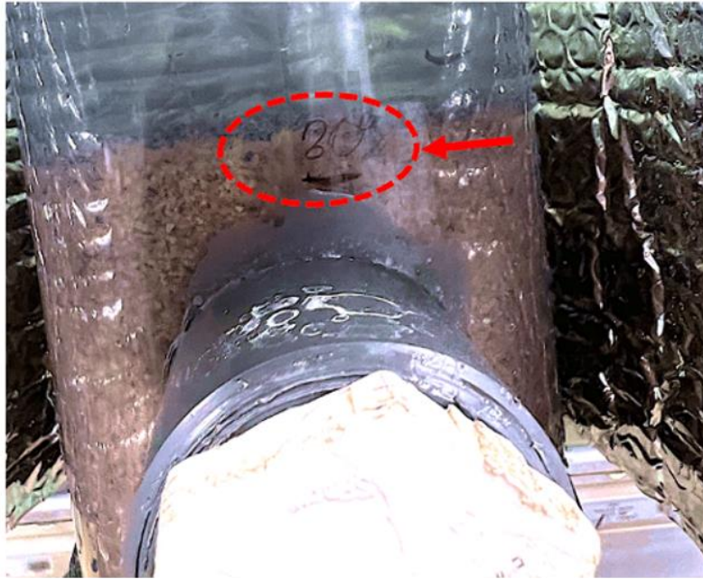
Figure A.10 Image highlighting the media expansion limit marking on the filter columns
