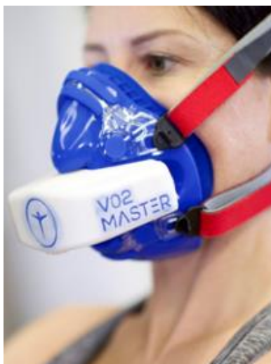
Figure 11: VO2 Master affixed to participant using a Hans Rudolph face mask. Figure retrieved from the VO2 Master Product Manual.
