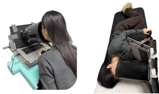
Figure 6. Upright and right side down (RSD) body orientations with the Oriented CHAracter Recognition Task (OCHART) laptop apparatus viewing tube.
