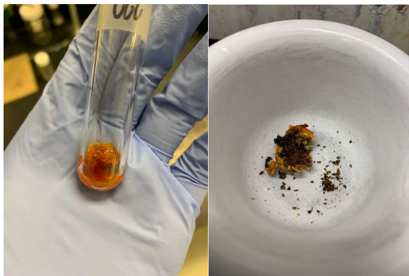
Figure 12: Product of the attempted phosphonylation of PVC using triethyl phosphite
