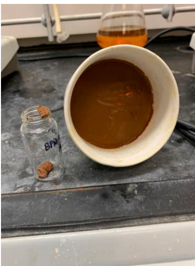
Figure 13: Product of the attempted phosphonylation reaction of PVC using the \text{Cs}_2\text{CO}_3 – promoted synthesis
