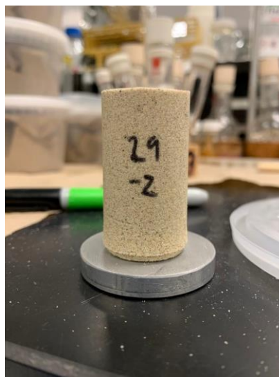
Figure 18: Samples made in the centrifuge tube moulds containing the slight taper in diameter towards the top
