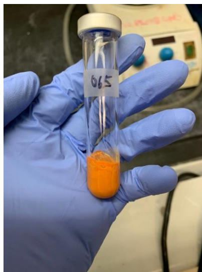
Figure 11: Product of the attempted phosphonylation of PVC using triphenyl and triethyl phosphite
