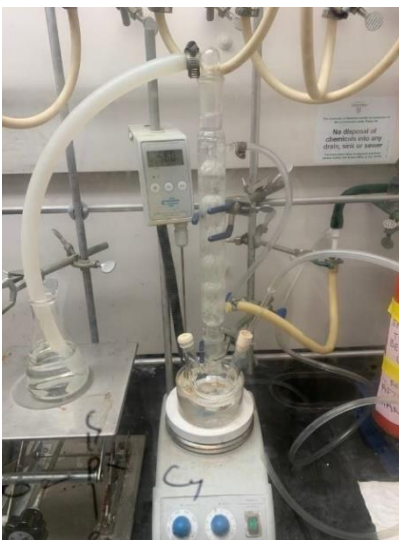
Figure 10: Attempted chlorophosphonylation of amorphous polypropylene
