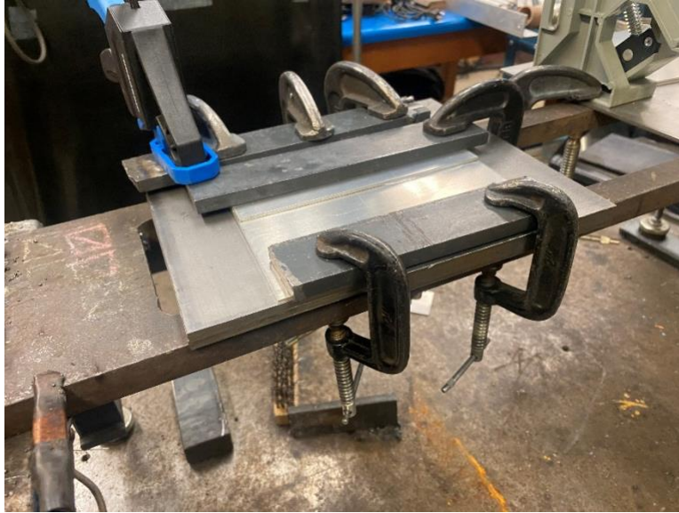
Figure 3-4: Lap joint fixture setup showing the two mating plates clamped rigidly with an overlap. The exposed edge of the top sheet is the location where the linear weld will be applied. Samples with dimensions shown in Figure 3-1 will then be waterjet cut from parent weld.
