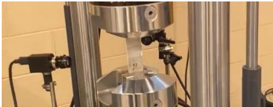
Figure 3-9: Camera setup for lap joint start and end recording during fatigue testing for crack initiation and propagation recording.
