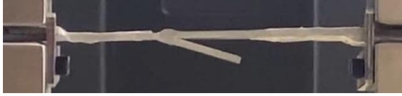
Figure 5-3: Lap joint eccentricity, with peel angle increasing with increasing applied load.
