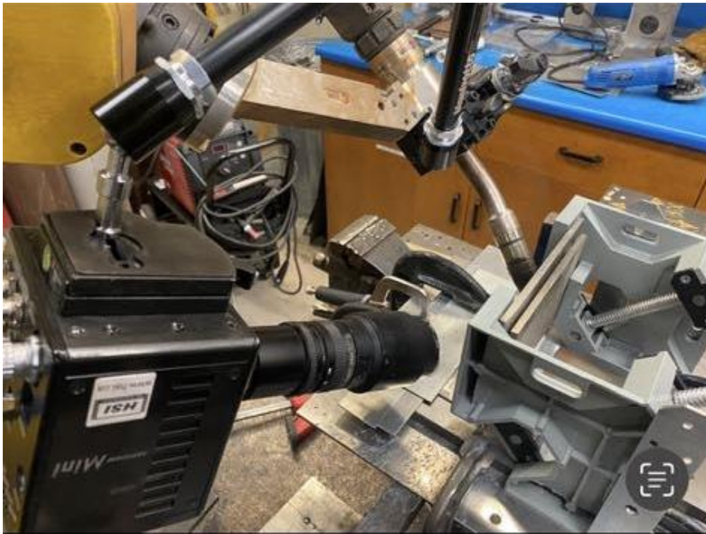
Figure 3-6: Welding high speed video setup. Camera is attached to the torch to maintain focus and lighting on the electrode.
