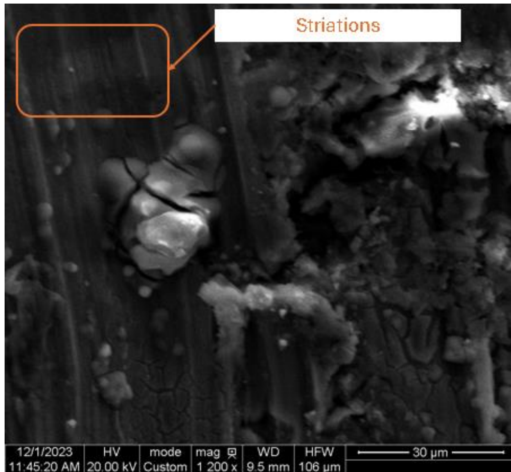
Figure 5-30: 1200X magnification of 10,000 cycle tee joint fractography showing possible striations emanating from the weld root area traveling across the thickness of the sample.
