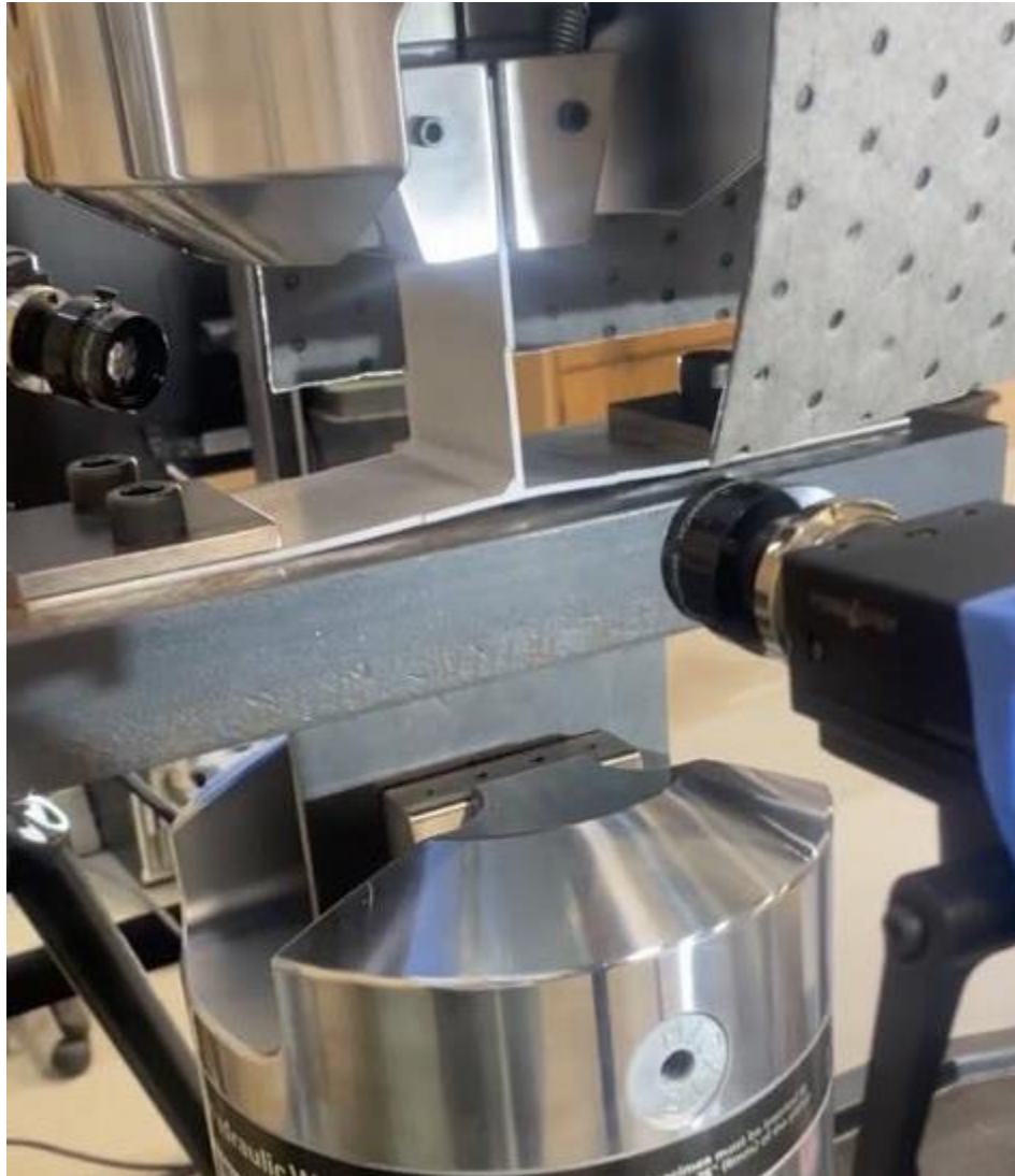
Figure 3-10: Camera setup for tee joint start and end recording during fatigue testing for crack initiation and propagation recording. Cameras are mounted on tripods for further stability during recording.
