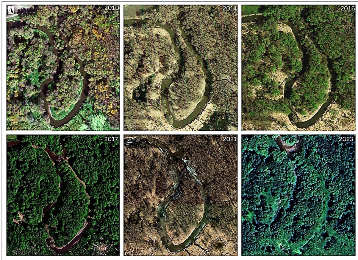
Figure 2: Meander Cutoff Evolution: an example of a neck cutoff formation in the Buffalo River, Minnesota, USA
