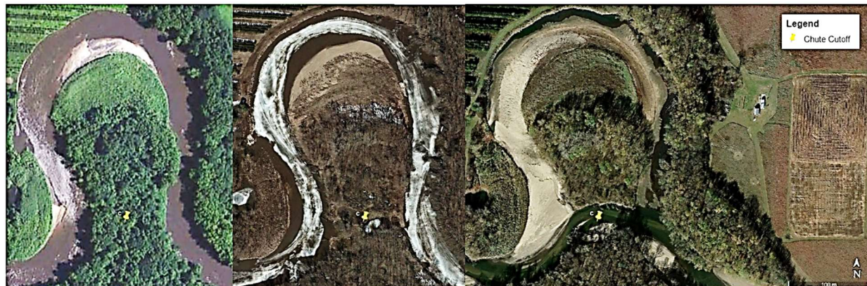
Figure 6: An example of the evolution of a chute cutoff in the Cedar River, United States (2011, 2015, 2020)
